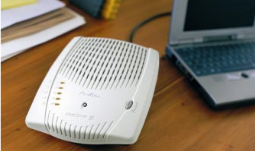
Figure 15 Ericsson currently offers two cable modem products: the PipeRider HM200c and HM201c. The HM200c is DOCSIS 1.0 certified and the HM201c is Euro-DOCSIS certified. The HM200c has received conditional @Home certification. The PipeRiders connect to customer premises equipment via USB and 10 Mbit/s Ethernet interfaces. A PipeLock security button allows the user to isolate the LAN and WAN sides of the cable modem when it is not in use, but keeps the modem attached to the system and available for instant access. In accordance with a specification in the DOCSIS standard, the modem software can be upgraded remotely by the cable operator. The HM200c/HM201c has been certified by regulatory bodies for use in the US, Canada, the EU, Japan, Korea, Australia, and China.
