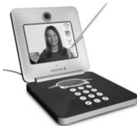
Figure 3 Prototype SIP telephone.
