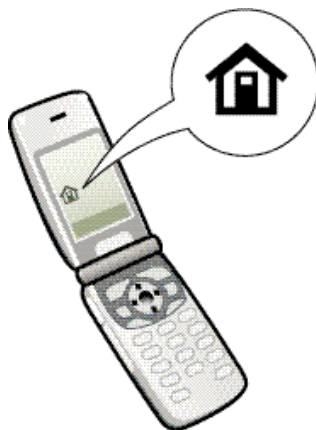
Figure 3 The handset displays a symbol to indicate that it is being served by the GAN.
