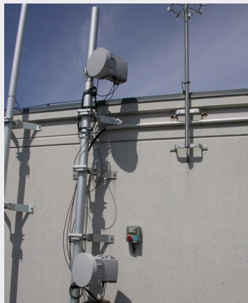
FIGURE 6 4x4 SS-DP LoS MIMO outdoor setup
