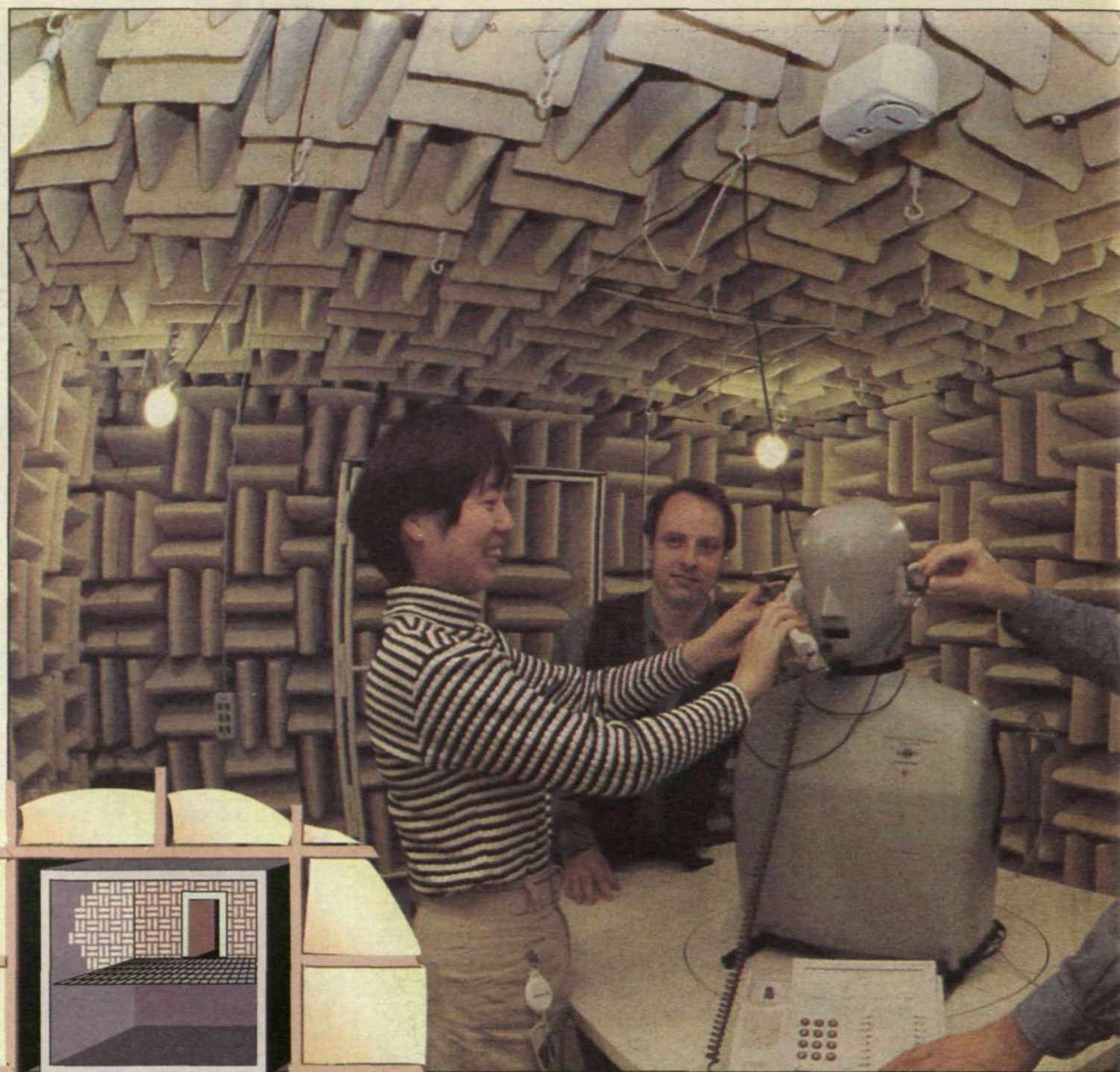
The Quiet Room measures 7.4 X 5.8 X 5.2 meters. It is made of concrete molded up to half of the height of the room, followed by concrete blocks up to the ceiling, which consists of plasterboard sheets. The room stands on springs that rest on a plate, which in turn stands on supports secured in bedrock. The Quiet Room, which represents an investment of SEK 1.7 million, was designed and built by G+H Montage, in Ludwigshafen, Germany.
