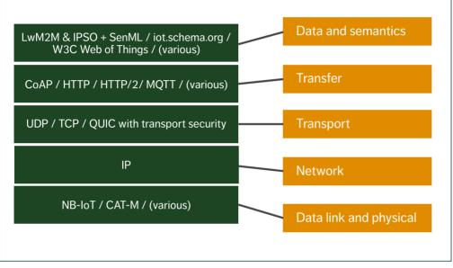
Figure 2 Structure of an IoT device protocol stack
