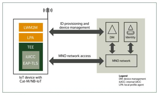
Figure 3 EAP-TLS ID management and use for network access
