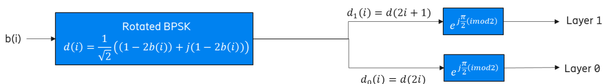
Figure 3-2: \pi/2 -BPSK modulation using the fixed two-layer transmission.
