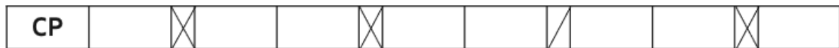
Figure 3-3 PT-RS design where group of four PT-RS samples (marked with the X) are mapped to the center of each of four intervals of data symbols, (also two or eight intervals is used, depending in the scheduled bandwidth).
