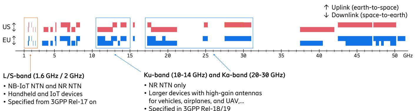
Figure 5: Spectrum allocations to satellite services in the EU and the US
