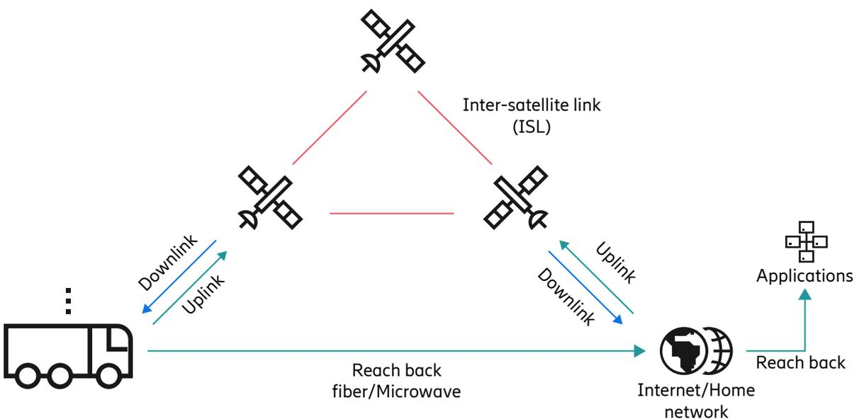
Figure 4: Backhaul deployable scenario
