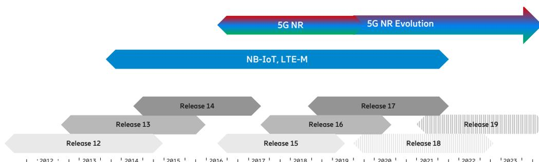
Figure 1 5G Timeplan and 3GPP Releases 12 to Release 19. NB-IoT and LTE-M are being evolved in 3GPP Release 17. The overlaps between the shown 3GPP releases are due to the fact that releases start with the services and system aspect (SA) studies roughly a year before the RAN specifications begin.
