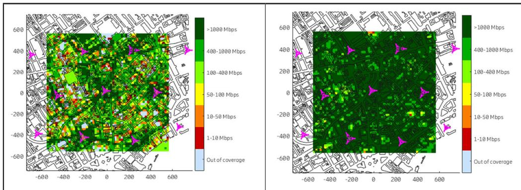
Figure 4 Efficient use of spectrum by combining different frequency bands.
