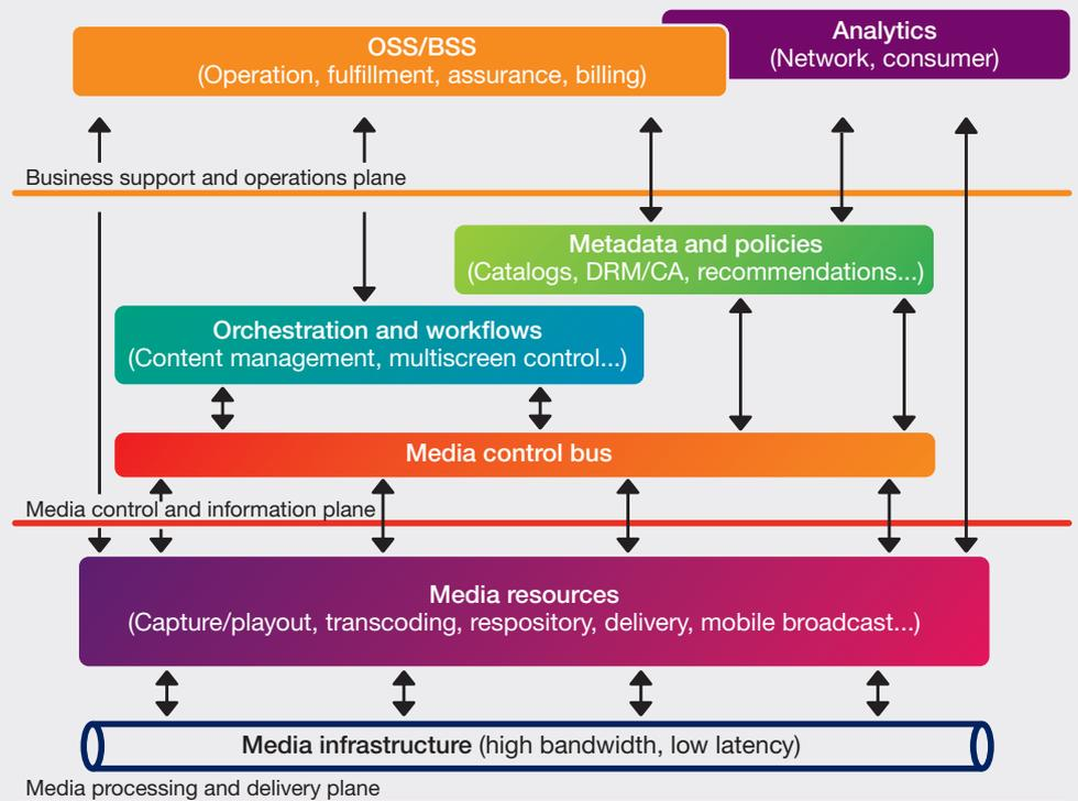
The media services architecture Ericsson has designed uses a component-based model. The resulting environment is loosely coupled; deployment- and integration-time-aware with self-contained functional components that are flexible (easy to replace or update) and reusable. Control is carried out through orchestration and workflows that determine which functions to invoke and when to invoke them in the content distribution and delivery process.
