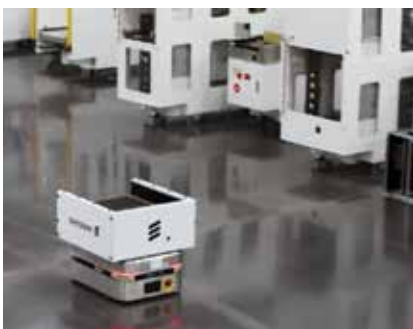
Figure 2: The AMRs provide material to multiple stations, depending on the current situation. (SOURCE: ERICSSON)
