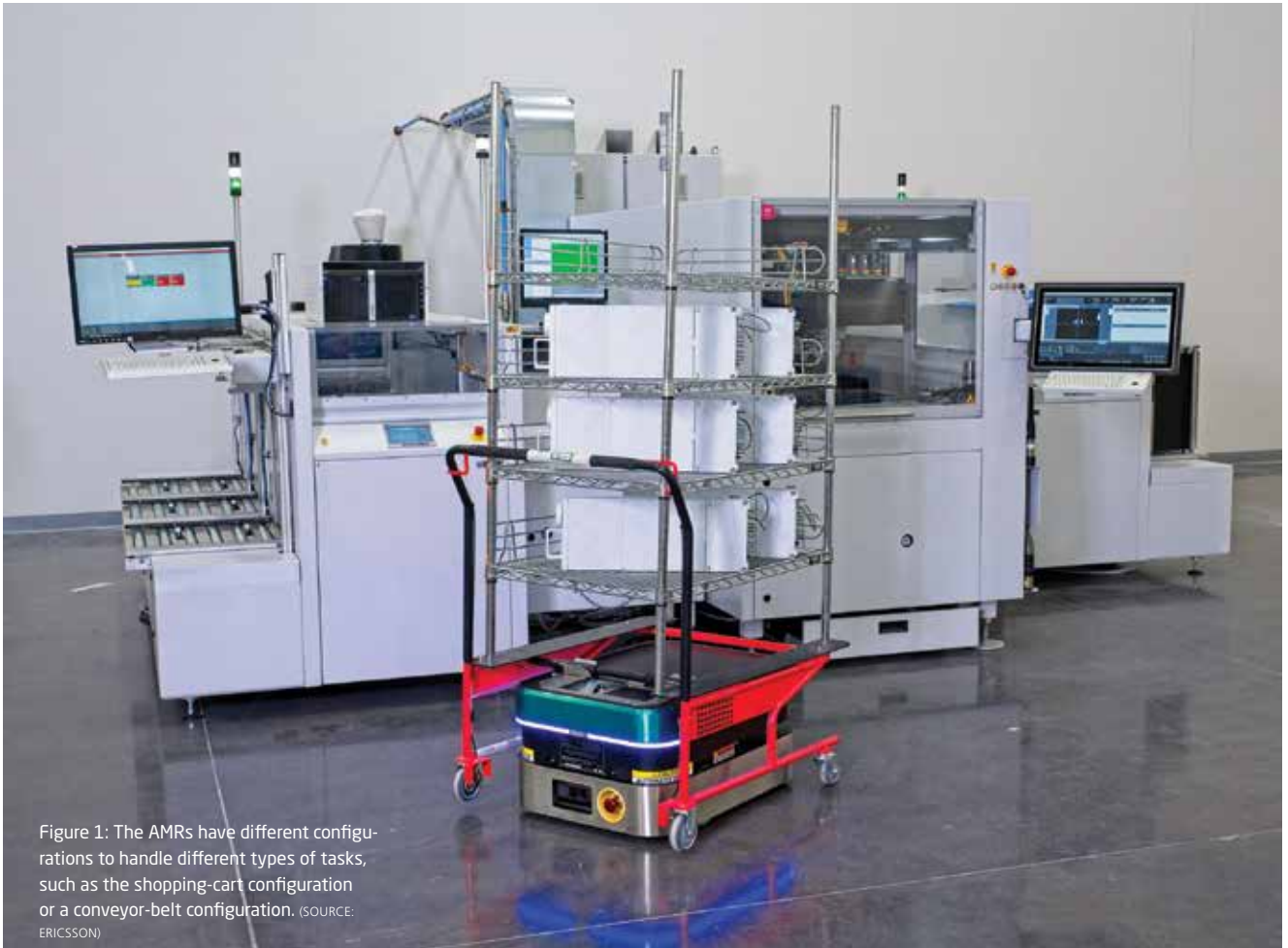
Figure 2: The AMRs provide material to multiple stations, depending on the current situation. (SOURCE: ERICSSON)
