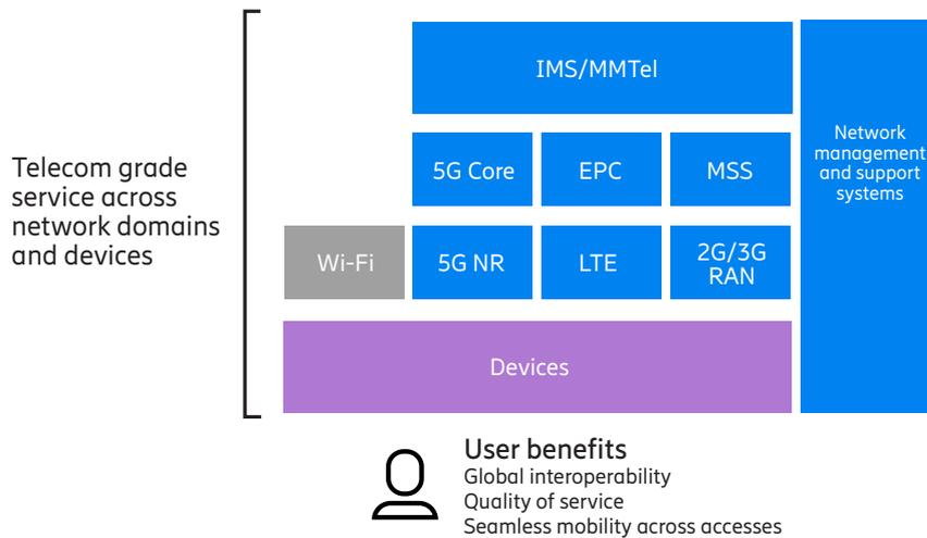
**Figure 1:** Overview of the telecom grade service across network domains and devices
