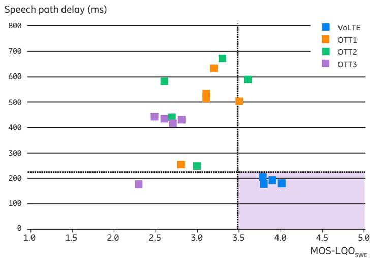
**Figure 3:** Voice quality test results in terms of MOS-LQOSWB and SPD for VoLTE and three OTT voice services during busy hours. The gray area represents the range for a high-quality voice service
