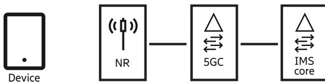
**Figure 5:** Communication services with NR and LTE as standalone access to 5GC
