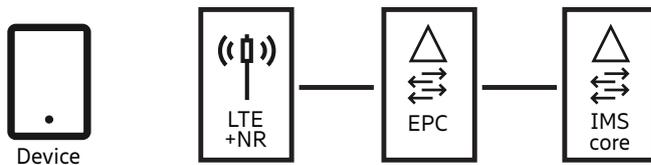
**Figure 4:** Communication services with LTE as standalone and NR as non-standalone access
