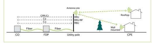
*Figure 8* Schematic figure of FWA showing CPE, antenna site, FDP and CO
