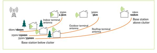
*Figure 7* Key findings on FWA feasibility for different scenarios and frequencies (3.5GHz cell ranges appear in bold text and 28GHz cell ranges in plain text)
