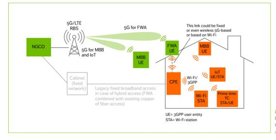
**Figure 1** Examples of FWA deployment alternatives
