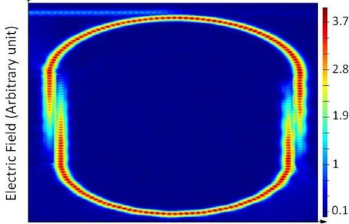
Fig. 2. FDTD simulation of the electric field in the broken racetrack at resonance.
