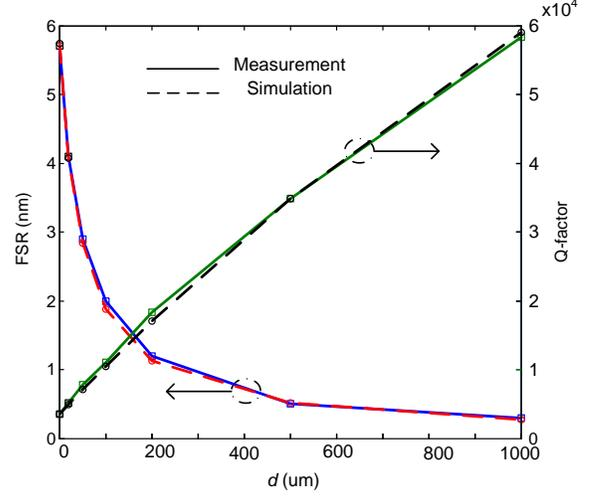
Fig. 6. Measured and simulated FSR and quality factor of the broken racetrack resonator versus displacement,  $d$ , based on 7 fabricated samples.
