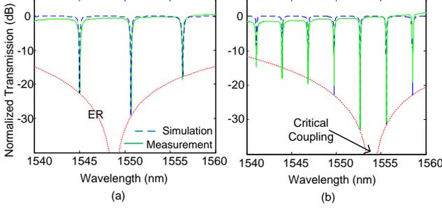
Fig. 5. Transmission response of the broken racetrack resonator for the displacement value of (a) 0 and (b) 50  $\mu\text{m}$ . The measured transmission response is in green and the response obtained from (2) is shown in dashed blue line. Extinction ratio is plotted in dotted red.
