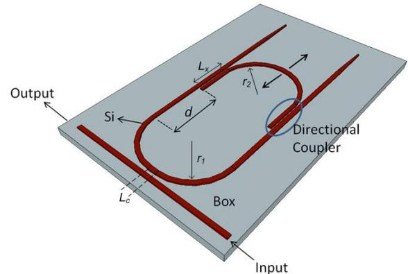
Fig. 1. Schematic diagram of the broken racetrack structure.  $d$  is the inner section displacement.
