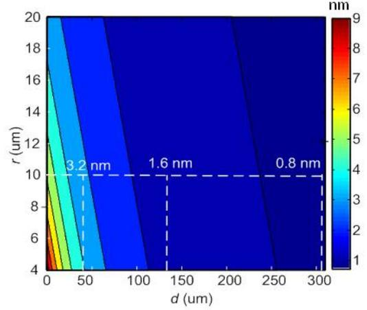
Fig. 3. FSR versus the racetrack radius and arm displacement.
