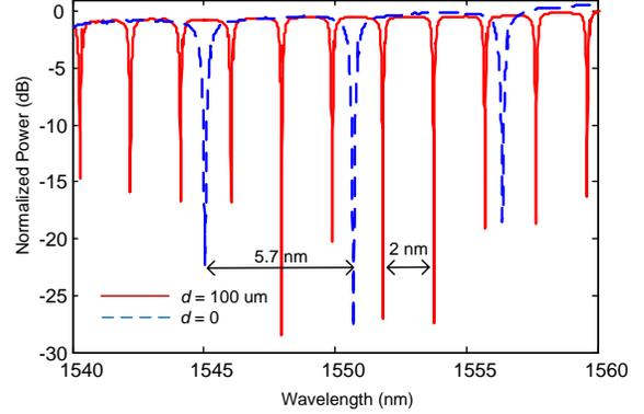
Fig. 4. Measured transmission response of the broken racetrack resonator for two displacement values of 0 and 100  $\mu\text{m}$ .
