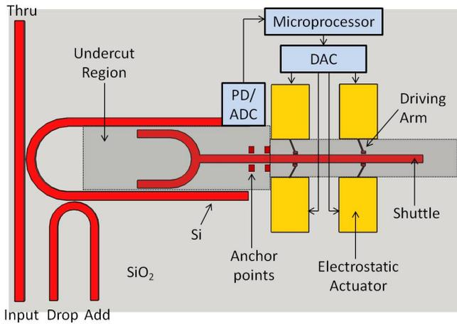
Fig. 7. Block diagram of the MEMS structure and the electronic feedback circuit. PD: photodetector, ADC: analog-to-digital converter. DAC: digital-to-analog converter.
