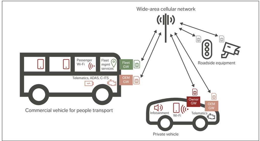
**Figure 2** Cellular connectivity for vehicles and roadside equipment
