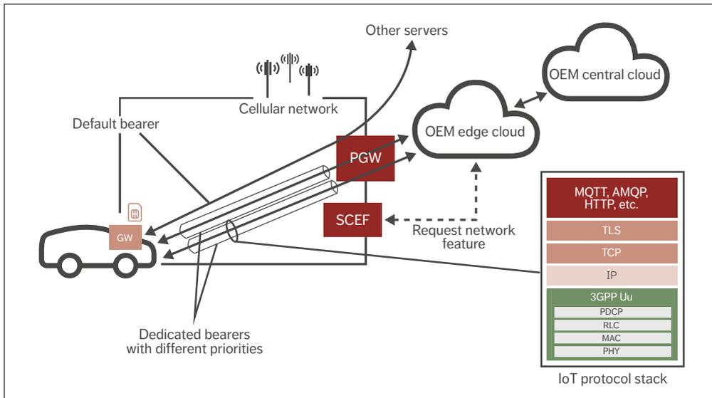
**Figure 3** Usage of dedicated bearers for traffic separation within one vehicle OEM cellular subscription
