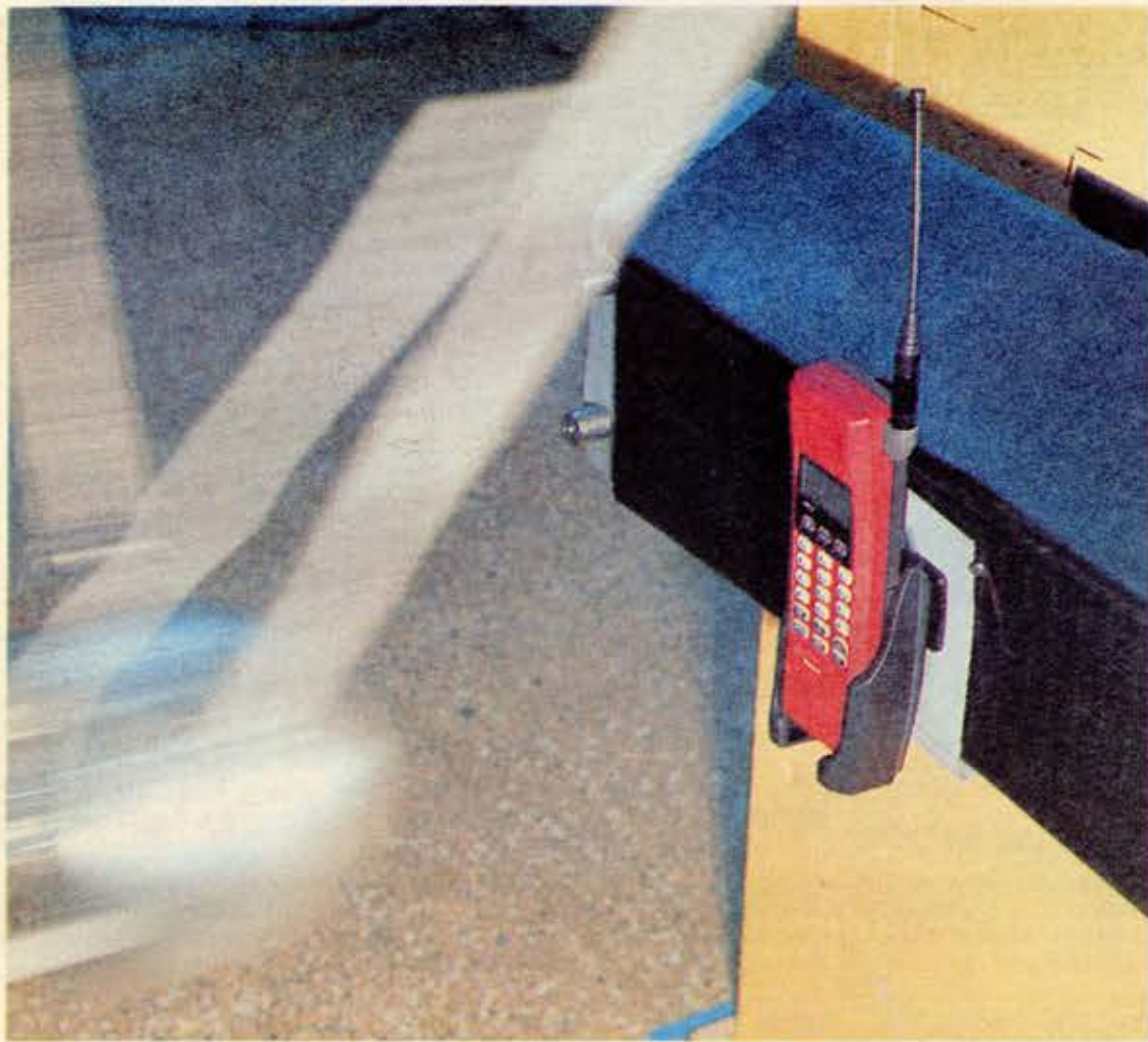
AT 24 km. per hour, the ball crashes into the car phone. The softer it lands the better. HotLine survived the test.
