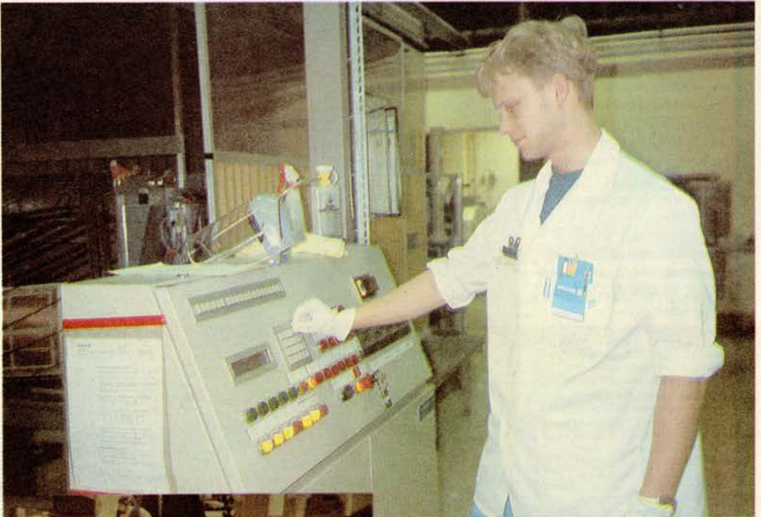
Christer Engdahl directs and monitors brown oxidizing of a printed board. This is done to achieve better adhesion of copper wiring.
