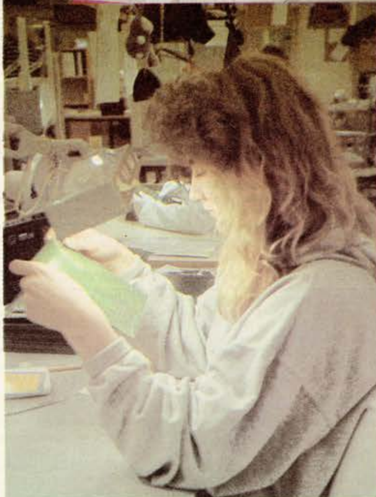
Ingela Gideonsson works with final testing, where she goes over the board manually. At this point electric tests are also done to make sure that all electrical parts are functioning.
