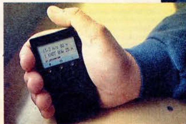
When an oil tanker has to berth at Scanraff's quay, north of Lysekil, they use people pagers. Through them, the pilot and two men on the quay get all the information they need. The vessel's speed and distance from the quay, current flow and current force.
