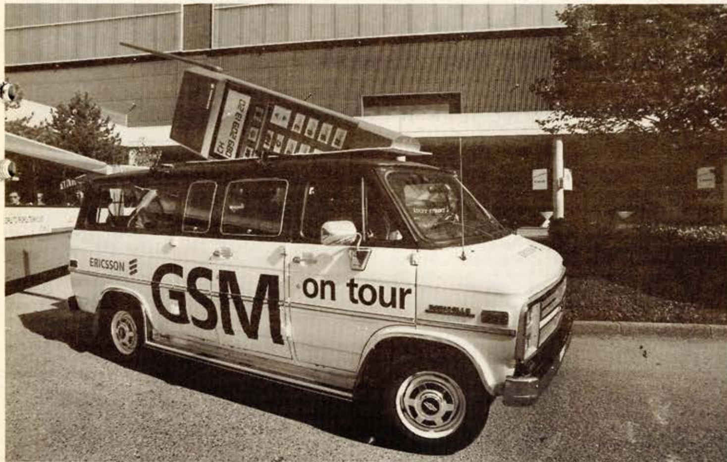
Ericsson had a demo car for the new pan-European digital mobile telephone system GSM, where it demonstrated handover and international roaming, that is what happens when you cross national boundaries.
