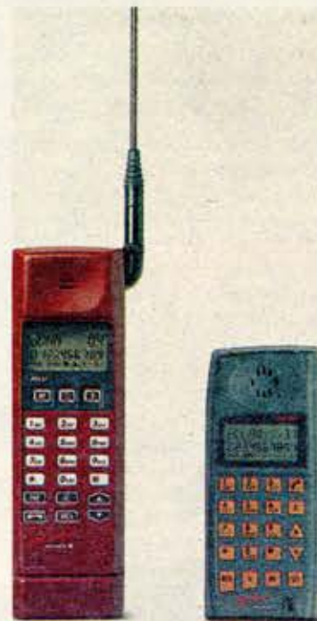
The new digital HotLine phone is considerably smaller than today's analog model.
