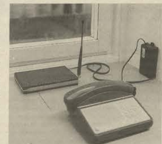
By connecting the ordinary telephone or fax to a radio unit, mobile telephones can be used to quickly provide telephone connections for business companies. Photo: Björn Seger
