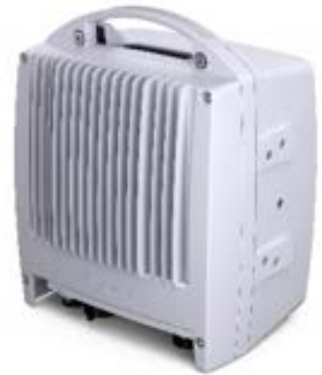
Figure 5: MINI-LINK 6352 E-band microwave
