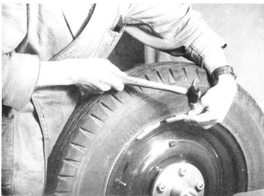
Fig. 5 The balancing weight is applied to the rim
