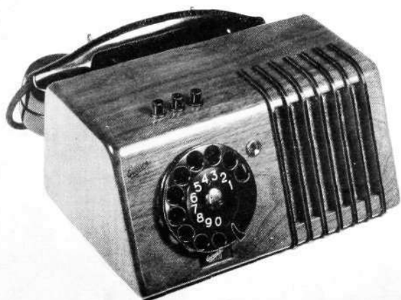
Fig. 1 X 7567 Telephone instrument type DBF 11 with built-in microphone. On the top of the instrument: push buttons, on the front: dial, pilot lamp and microphone; (right) rear view
