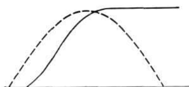
Fig. 7 X 4659 Comparison between a lightning current and a sinusoidal current with approximately the same derivative \frac{dI}{dt}
