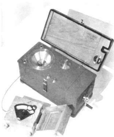
Fig. 3 X 4682 Carbometer for determining the carbon contents in a steel bath
