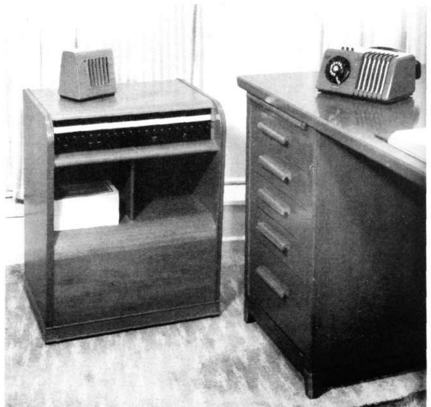
Fig. 3 Conference telephone (left) Manager's table and loudspeaker, (right) On the desk the new telephone instrument with built-in microphone
