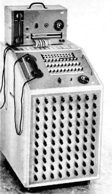
Fig. 6 X 2066 Traffic route tester with portable receiver unit placed on top of transmitter unit
