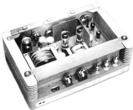
Fig. 4 Amplifier unit ZGA 3901 rear view with cover removed
