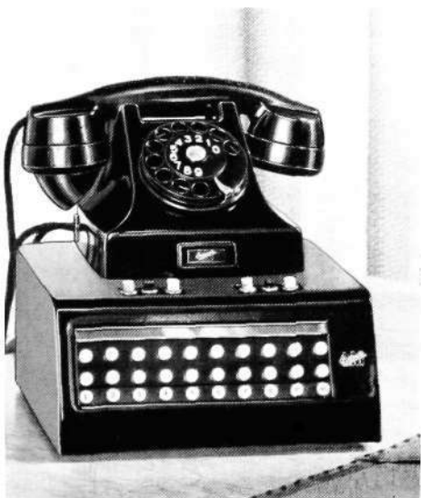
Fig. 4 X 2042 Manual line connection set for 10 (12) lines
