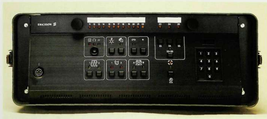
Fig. 3 The operator panel constitutes the front of the exchange
