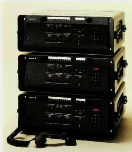
Fig. 2 Up to three ABM 301 can be connected together to form a larger exchange
