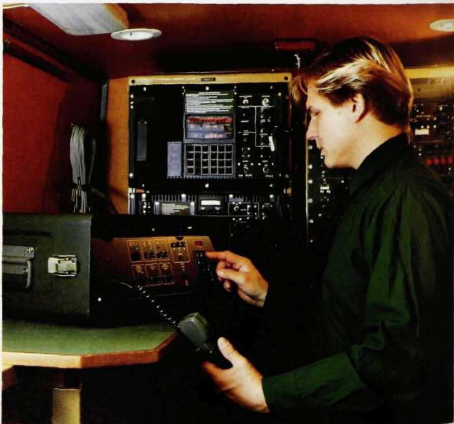
Fig. 1 Automatic field telephone exchange ABM 301 for 12 extensions and three trunk lines
