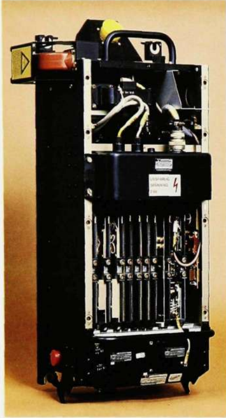
Fig. 4a The illuminator with the cover removed. The klystron is placed at the top, with the high-voltage parts and electronic circuits on printed boards below
