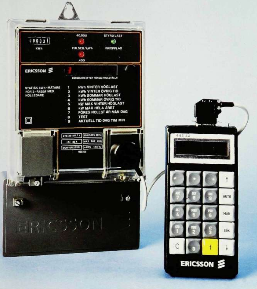
Fig. 5 The meter-reading terminal is connected to a panel in the bottom right-hand corner of the meter. The coupling is by means of a magnet and a metal plate
