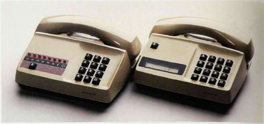
Fig. 7a Multi-line system with access to all trunk lines
