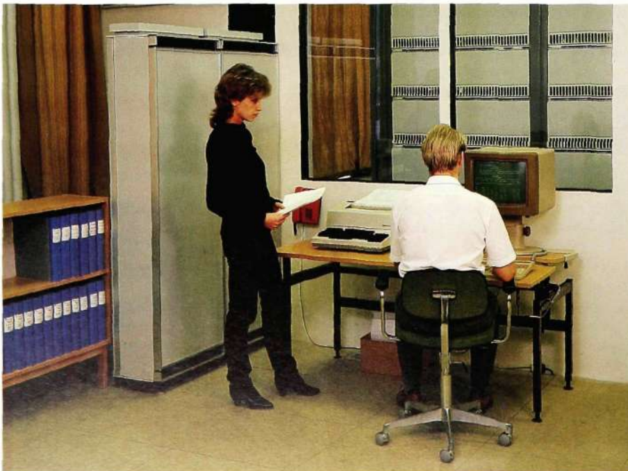
Fig. 5 TRTC uses BYB cabinets holding five magazines each. The I/O equipment consists of a visual display terminal and a printer
