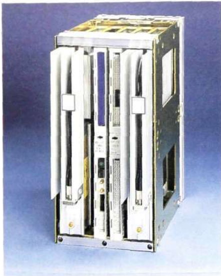
Fig. 5 Two-way intermediate repeater for 565 Mbit/s. Thanks to a high degree of integration it has been possible to build a very compact unit containing two transceiver units, one fault detector unit and one d.c./d.c. converter. The width is 122 mm, the height 244 mm and the depth 220 mm
