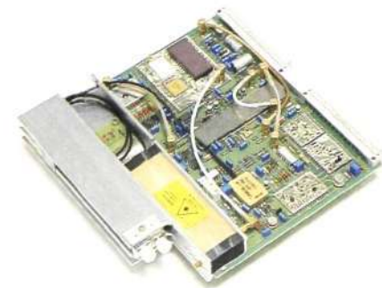
Fig. 6 On the 565 Mbit/s transceiver board all high frequency signal processing employs hybrid circuits developed by Ericsson and manufactured by RIFA AB, a member of the Ericsson Group. The picture shows a transceiver unit with the screening of the hybrids removed. The laser unit with internal control of temperature and working point is mounted at the front of the board
