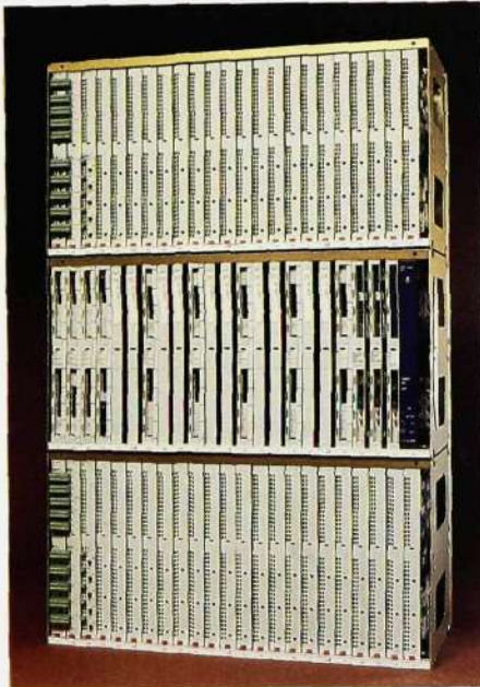
Fig. 11 ZAJ 120-3, transmultiplexer for 120 channels
