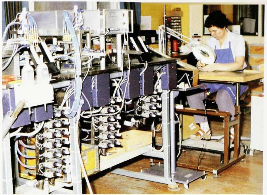
Fig. 7 The last part of the assembly line. The operator carries out visual inspection of the soldering and packs the keyboards
