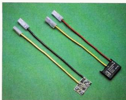
Fig 7 Cell voltage equalizers in hybrid technique. One equalizer is shown before encapsulation. The components are surface-soldered on to a ceramic substrate
