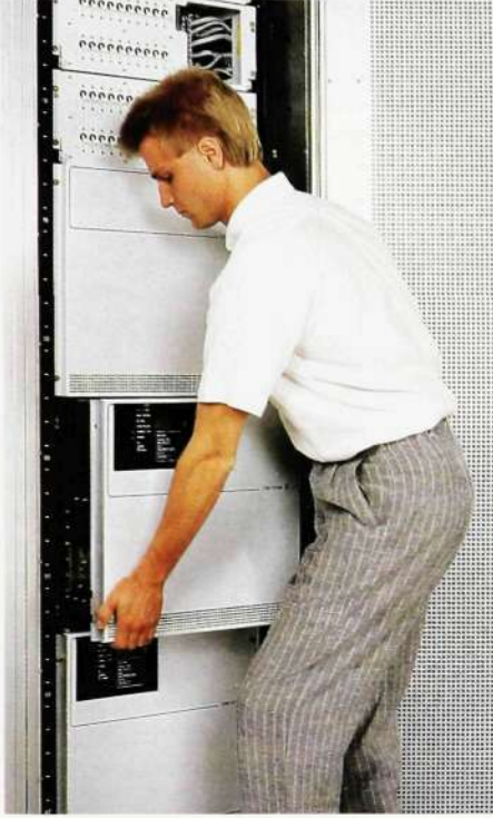
Fig 4 Units can easily be replaced by one man during operation
