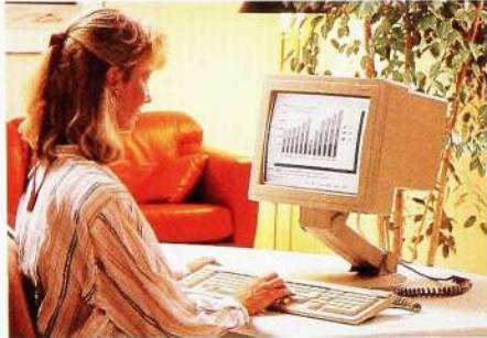
Fig. 3 VDU with a positive screen, i.e. dark characters on a light background
