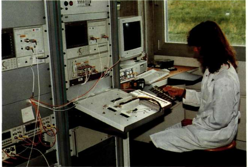
Figure 12 Test equipment (at Valtronic, Les Charbonnières, Switzerland) consisting of two joined instrument cabinets with a protruding operator's test table and a PC with a bar code reader.
