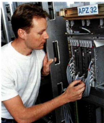
Figure 6 The APZ 212 25 occupies only half a subrack in the BYB 501.
