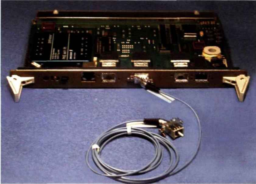
Figure 2 EriOpto4 mounted at the front of a printed board assembly.
