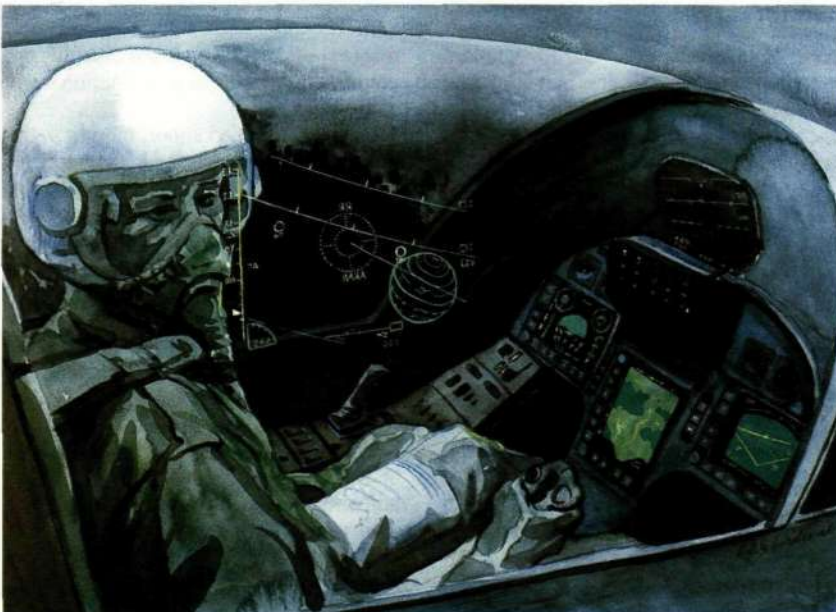
Figure 9 In a fighter aircraft, the pilot uses HMD presentation together with other displays on the instrument panel. Important information is always displayed in front of his eyes. He can also point out targets to the HMD by placing a displayed marker in the respective target positions.
