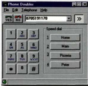
Figure 5 The Phone Doubler client permits users to make, answer and reject calls. The client window pops up on the screen when an incoming call is on the line.
