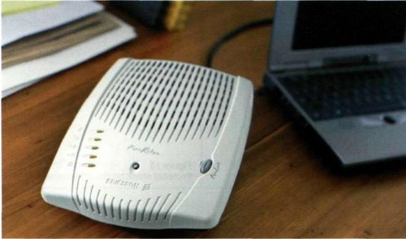
Figure 15 Ericsson currently offers two cable modem products: the PipeRider HM200c and HM201c. The HM200c is DOCSIS 1.0 certified and the HM201c is Euro-DOCSIS certified. The HM200c has received conditional @Home certification. The PipeRiders connect to customer premises equipment via USB and 10 Mbit/s Ethernet interfaces. A PipeLock security button allows the user to isolate the LAN and WAN sides of the cable modem when it is not in use, but keeps the modem attached to the system and available for instant access. In accordance with a specification in the DOCSIS standard, the modem software can be upgraded remotely by the cable operator. The HM200c/HM201c has been certified by regulatory bodies for use in the US, Canada, the EU, Japan, Korea, Australia, and China.
