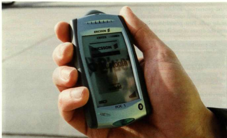
Figure 1 This future, pocket-sized, mobile multimedia concept device features voice, imaging, and video. A wireless, hands-free ear-phone connects via a Bluetooth connection.
