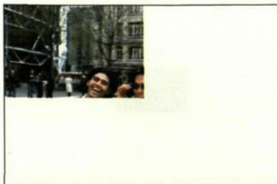
Figure 9 Progressive by position. The image is encoded in scan-line order so that the recipient first gets the top-left region of the image at full quality and resolution; the recipient then receives the remaining parts of the image from left to right and from top to bottom.
