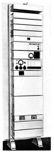
Fig. 5 X 2306 Line Amplifier Bay for an auxiliary repeater station
