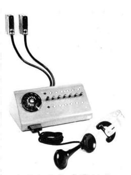
Fig. 1 X 2371 Multi-line telephone AEA 1121 with headset
