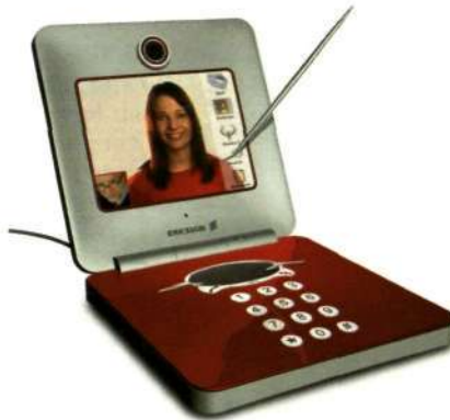
Figure 3 Prototype SIP telephone.
