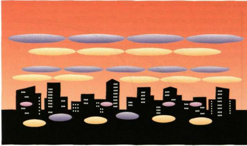
Figure 2 Network capacity: Efficient traffic-management features, such as Ericsson's multilayered hierarchical cell structure (HCS), should be employed when different kinds of cells and frequency bands are used.
