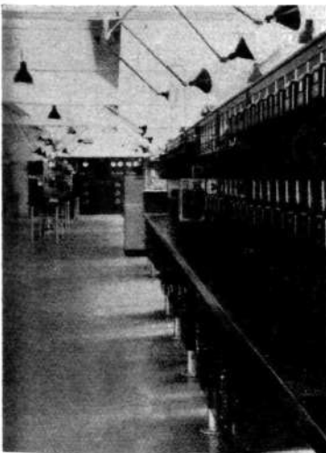
Fig. 1 Ericsson's testing department for electricity meters Right, testing board for single-phase meters; in background, testing board for DC meters and instrument board
