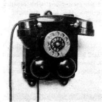
Fig. 10 Watertight automatic wall instrument
