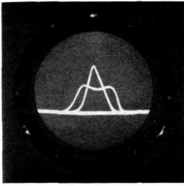
Fig. 4 X 3526 Amplification as function of frequency for intermediate-frequency amplifier, obtained in cathode-ray oscillograph for maximum and minimum selectivity
