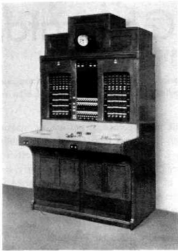
Fig. 2 Two-position operator's desk at police station
