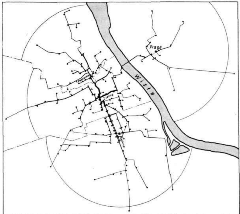
Fig. 4 X 5198 Primary cable network in Warsaw
