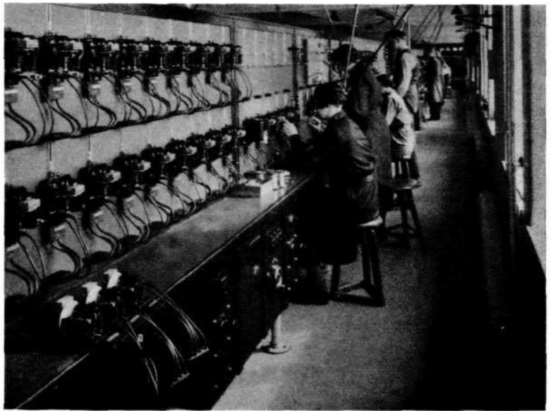
Fig. 2 Testing board for single-phase meters The meters are fixed to the board and connected up by a simple operation
