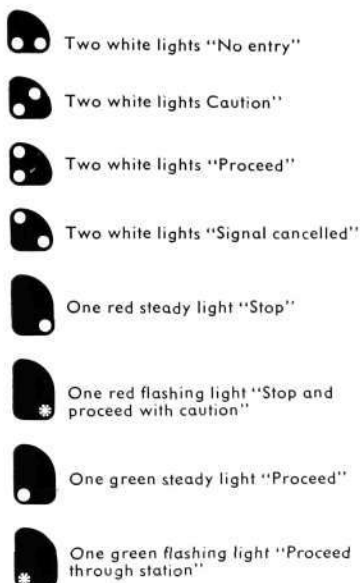
Fig. 2 Schematic survey of signal concepts which can be displayed from dwarf and platform exit signals.
