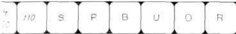
Fig. 4 Keypad for key-base DYA II S Secretary P Post B Messenger U Engaged O Switching key R Restore key
