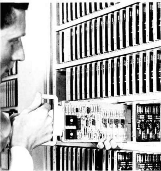
Fig. 11 Printed Circuit Card in the Transfer Unit
