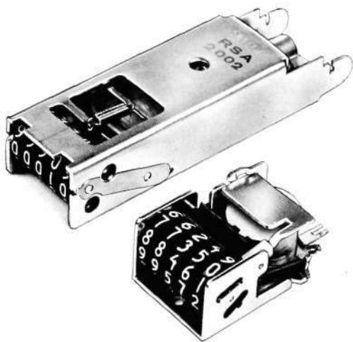
Fig. 20 New RSA subscriber meter In the background the type employed hitherto
