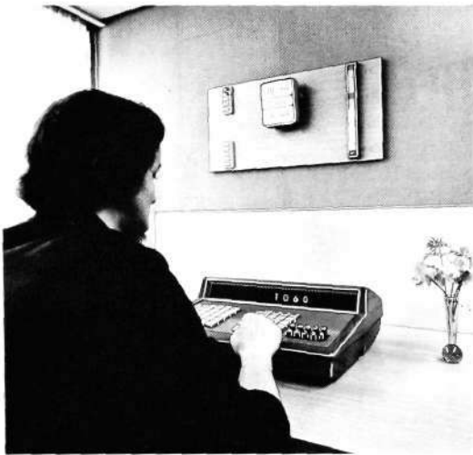
Fig. 3 Queue "thermometer" visibly placed on the wall in front of the operators. On the same panel there is also a time-and-date clock and two lamp panels.
