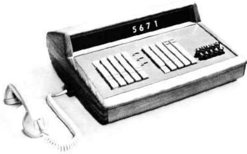
Fig. 2 Operator's console with numerical indication of called extension
