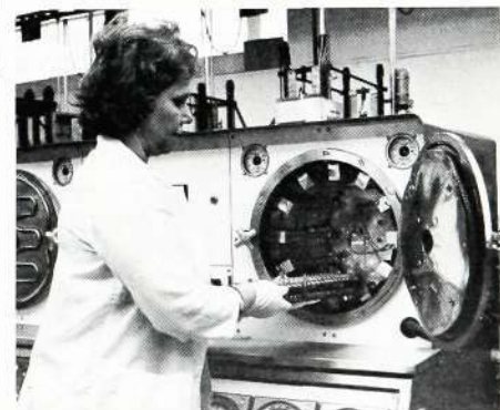
Double-furnace equipment for vacuum pumping, gas filling and soldering of transient voltage protectors at the Rifa factory at Bollmora outside Stockholm.
