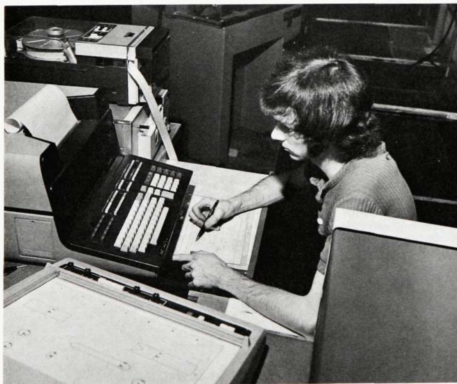
In the workshop specially trained workshop staff carry out programming of punched tape for the numerical control of, for example, wire spark machines, using electronic calculators
