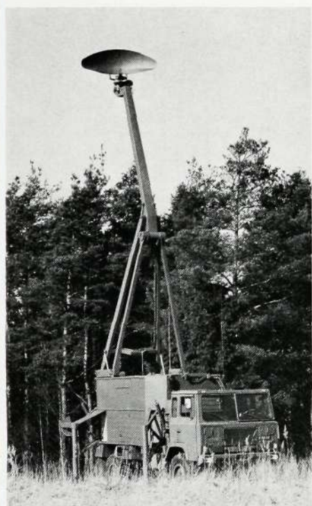
The prototype of the L M Ericsson mobile search radar PS-70/R which was developed for the new anti-aircraft robot system of the Swedish army, has been delivered to the Material Administration of the Swedish Armed Forces. PS-70/R is a pulse-Doppler radar that distinguishes between echoes from fixed and moving objects and which can track approaching enemy aircraft even at treetop level. The picture shows the equipment mounted on a cross-country lorry
