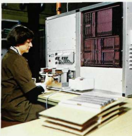
Fig. 9 Microprocessor-controlled equipment for the final electrical testing of reed switches that are ready for delivery. The switches are tested with regard to operational reliability, test currents, speech path resistance, double operation, unwanted release and dielectric strength
