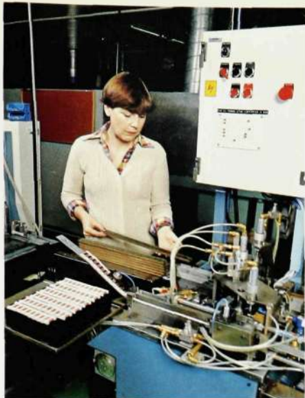
Fig. 5 Equipment for assembling cross point relays
