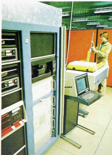
Fig. 8 Minicomputer-controlled equipment for testing the static and dynamic parameters of micro circuits. It is used for the acceptance inspection of the micro circuits for the reed switch
