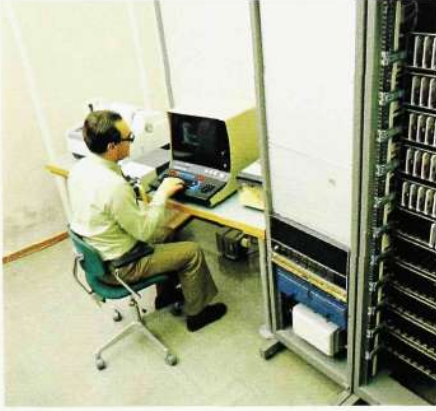
Fig. 7 Minicomputer-controlled equipment for electrical endurance testing of reed contacts. The equipment permits simultaneous testing of 50 reed contacts under conditions that can be varied as regards frequency, contact closure time, contact break time, current, voltage and type of load (resistive, inductive or cable). The contact resistance is measured and the release time is checked for each contact operation
