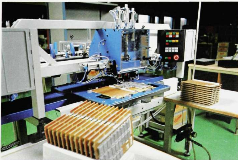
Fig. 6 Numerically controlled equipment for the automatic mounting of cross point relays on printed boards. The equipment places the required relays on the board and then bends the soldering and fixing tags on the back of the board
