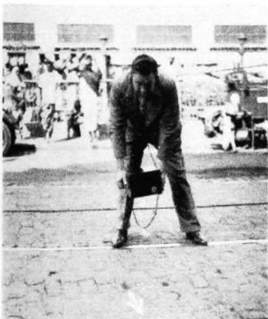
Fig. 3 Determining by the null method the exact position of a cable
