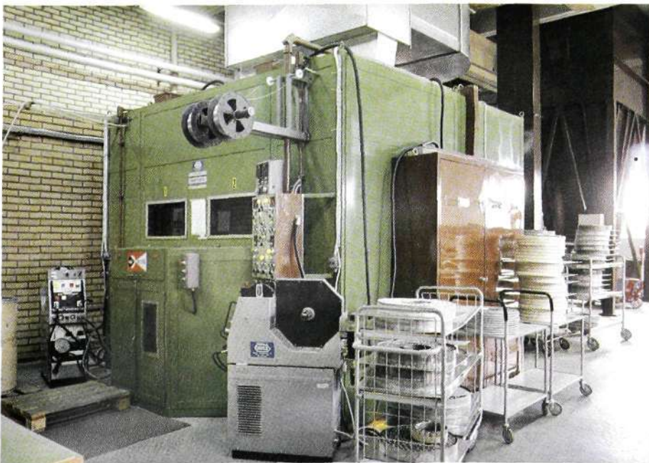
Fig. 10 The capacitor ends are sprayed in specially designed metal spraying equipment
