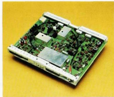
Fig. 5a APD receiver. The phase-locked loop is built up around a voltage controlled crystal oscillator, which ensures low output jitter
