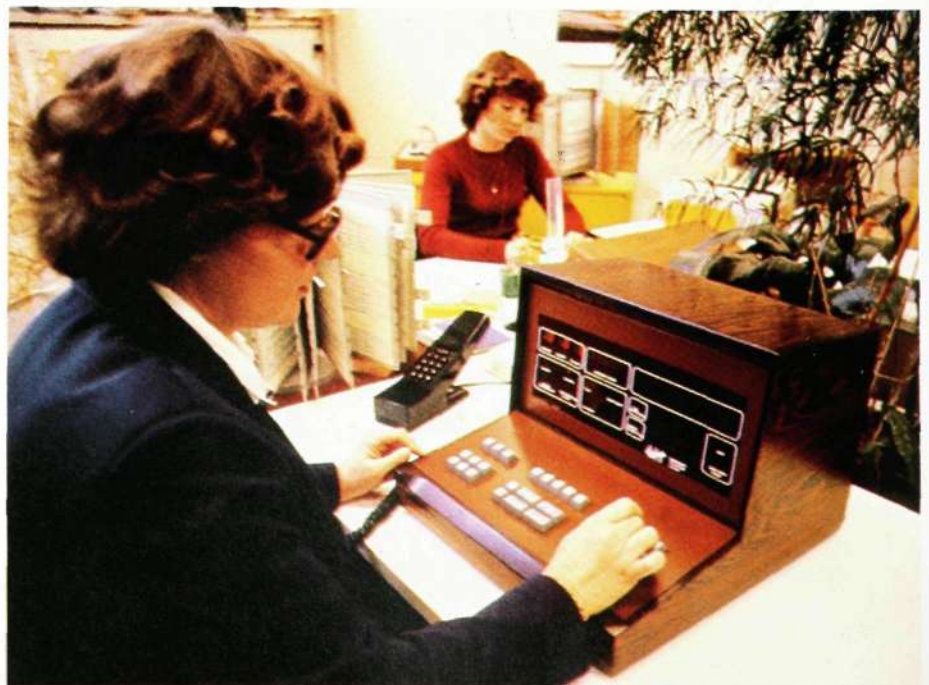
Fig. 3 The operator's unit used for receiving emergency calls has a simple construction and is easy to handle
