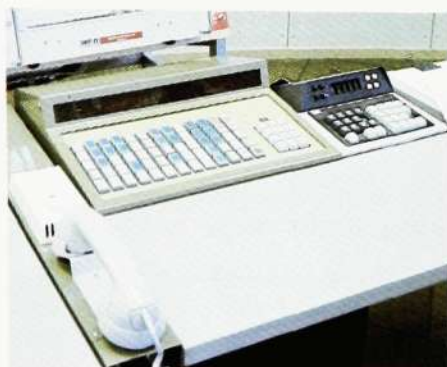
Fig. 2 To the right a key-set for controlling train traffic and to the left sets for different telephone systems
