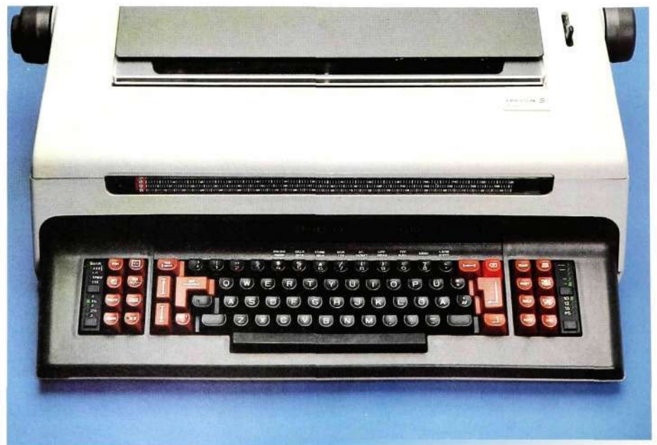
Fig. 6 The line display holds 40 characters, of which 34 are used for text and 5 for state information. The keyboard is of a low profile type and ergonomically designed. Approximately 300 characters can be obtained by means of different key combinations
