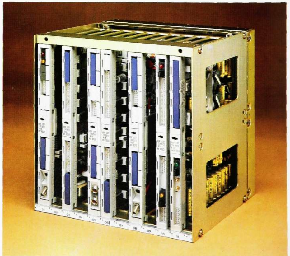
Fig. 7 The line terminating magazine is built up in a BYB magazine, with the connectors at the front of the units
