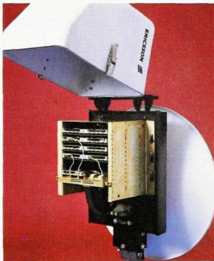
Fig. 5 The magazine with the printed board assemblies installed
