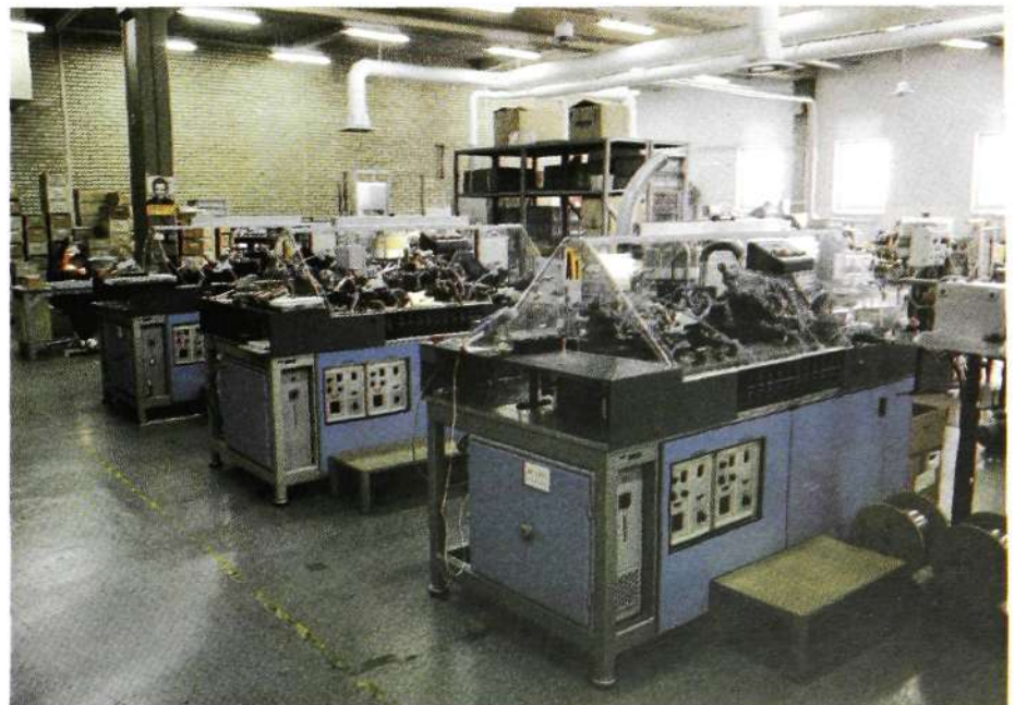
Fig. 13 Like most other machines used in the production process the braze welding and assembly machines have been designed and manufactured by RIFA
