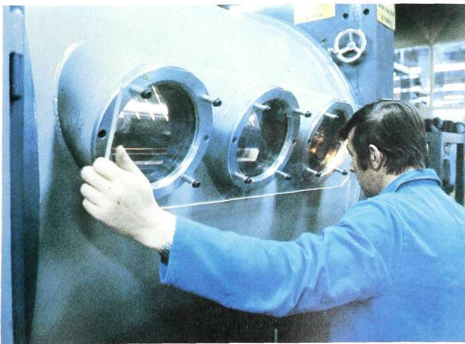
Fig. 6 Supervising the metallizing process
