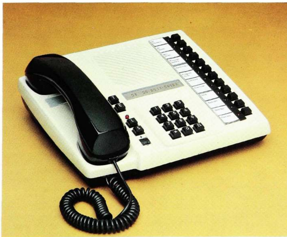
Fig. 15 Digital system telephone. A larger version with 36 programmable function buttons is also available
