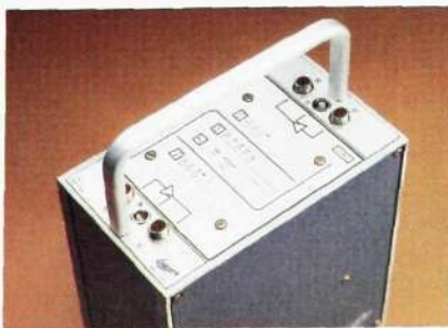
Fig. 12b The cover of the repeater holds the four coaxial line cable connectors and the two connectors for the fault location equipment. The top cover of the repeater also serves as a label where the chosen settings can be recorded
