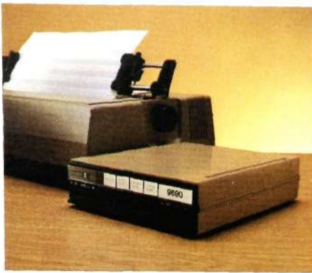
Fig. 8 Data circuit terminating equipment DCE-S
