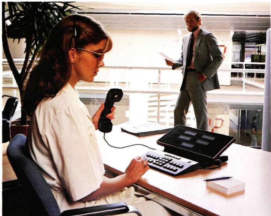
Fig. 1 The operators keyboard and visual display unit are separate units in MD 110
