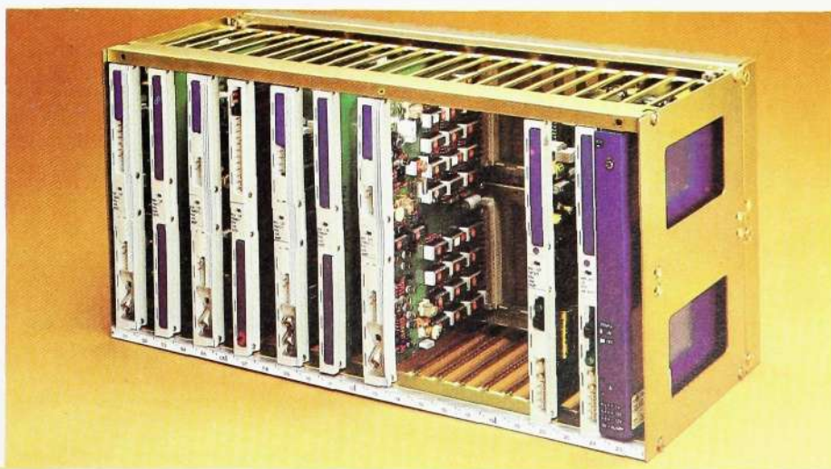
Fig. 3 The line terminating magazine where recoding, jitter reduction and supervision are carried out
