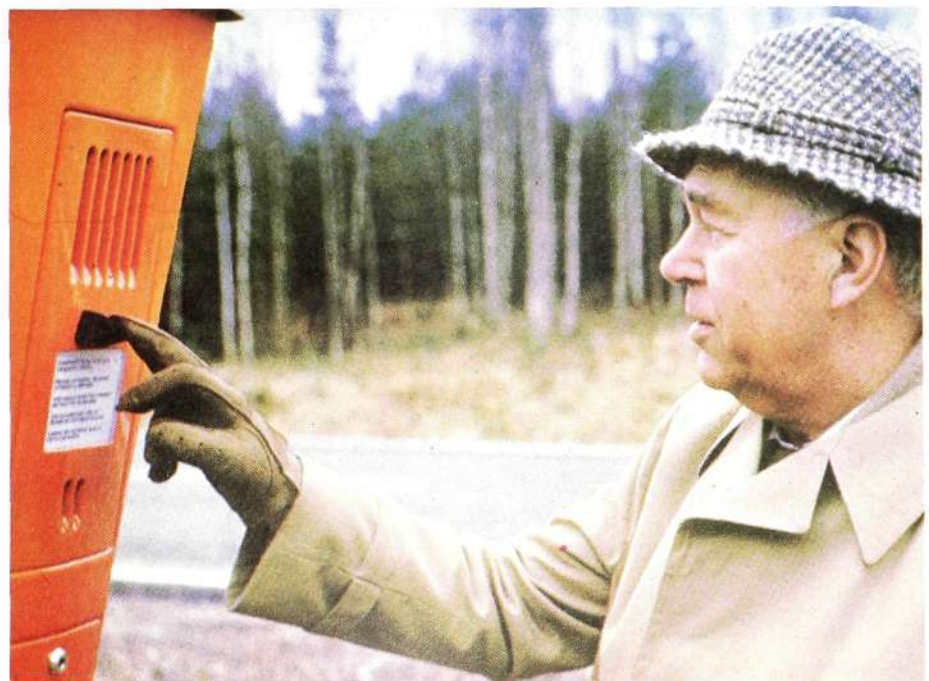
Fig. 4 The emergency telephone is easy to operate. The caller only has to turn the calling handle. When the operator answers the call a two-way loud-speaking connection is set up
