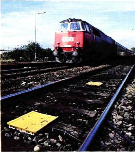
Fig. 16 Optical fibre beacon installed at a beacon site which contains two beacons
