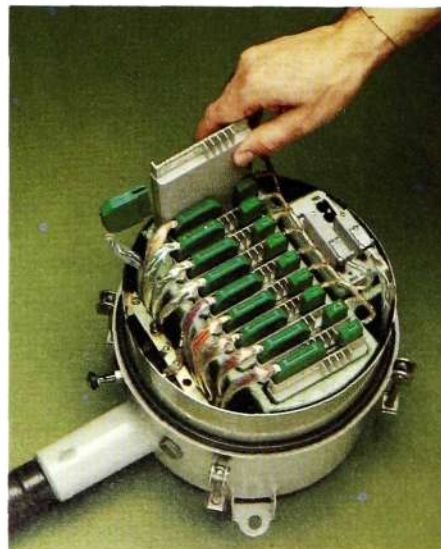
Fig. 8, left Housing ZDD 53601 with the top removed. Holds 10 two-way repeaters for ZAD 0.7-1, ZAD 2-4 or ZAD 2-5. Dimensions: \varnothing 260 mm, h = 320 mm. Weight: approximately 24 kg when fully equipped, including the stub cable
