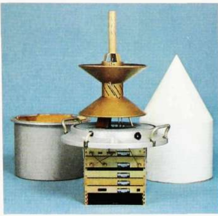
Fig. 19 AGA-ERICON equipped with the S-band subunit and side lobe memory
