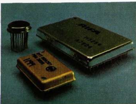
Fig. 15 Hermetic encapsulation for military use
