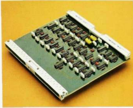
Fig. 10 A control unit for ZAK 480/1920 equipped with ECL components. Multi-layer printed boards have been used in order to obtain impedance-matched connections between the components
