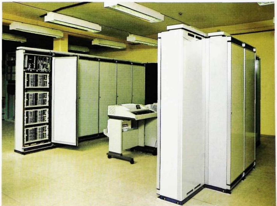
Fig. 2 The LM Ericsson computer UAC 1610 P for stored program control of the signal box for the Malmö railway yard area, in south Sweden
