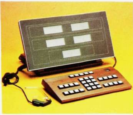
Fig. 8 MD 110, a new stored program controlled PABX for voice and data. The system has a modular structure and can be extended to 10 000 extensions
