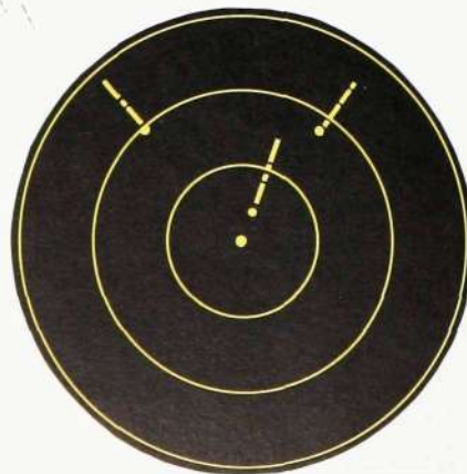
Fig. 22 When navigating by radar in areas where oil is being extracted it is often difficult to orientate oneself and identify specific targets. Ships at anchor and fixed platforms give similar echoes on the radar indicator. The relative positions of different installations can change from one visit to the next. Racons with different response codes installed on stationary platforms give easily identifiable reference points and reduce the risk of disastrous navigational errors. In the case of a gas leak or other dangerous situations on a platform a racon with a specific response code can warn approaching ships
