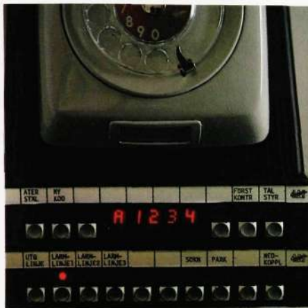
Fig. 7 Four figures show the identity of the person sending the alarm. The letters A–F give the type of alarm
