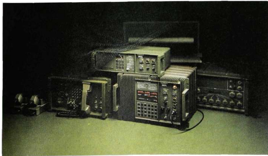
Fig. 8 Radio relay equipment CONTACT RL420 with field telephones, bulk encryption equipment, digital multiplexors and digital node switches are some of the units that are now available for building up digital encrypted telephone networks
