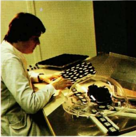
Fig. 12 Final testing of speech circuits
