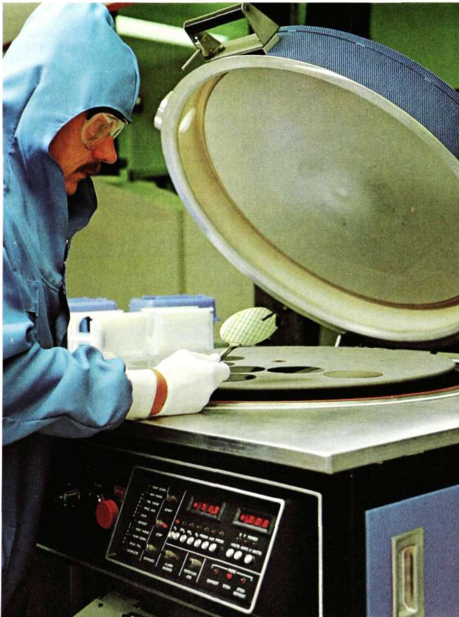
Fig. 4 A plasma nitride reactor. The last layer, on top of the aluminium conductor pattern, consists of a silicon nitride layer, which protects the circuit better than an oxide layer which has been deposited in the conventional way at a low temperature (vapox, silox). This increased protection is very important for circuits which are to be encapsulated in plastic
