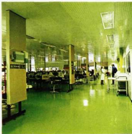
Fig. 3 The department for assembly of chip & wire circuits. The subdued lighting is specially adjusted for microscopy
