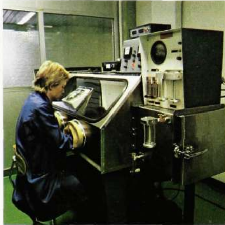
Fig. 16 The package welding takes place in a glove box containing pure nitrogen
