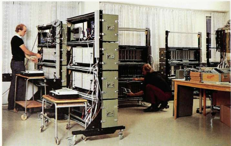
Fig. 12 Calibration of stored program controlled traffic generators in the MIPSC unit dealing with test equipment
