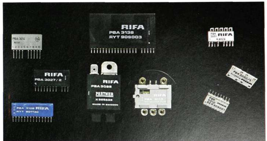
Fig. 10 After encapsulation and cutting of the leads to the correct length the circuits are ready for the final testing. The figure shows various types of encapsulated circuits
