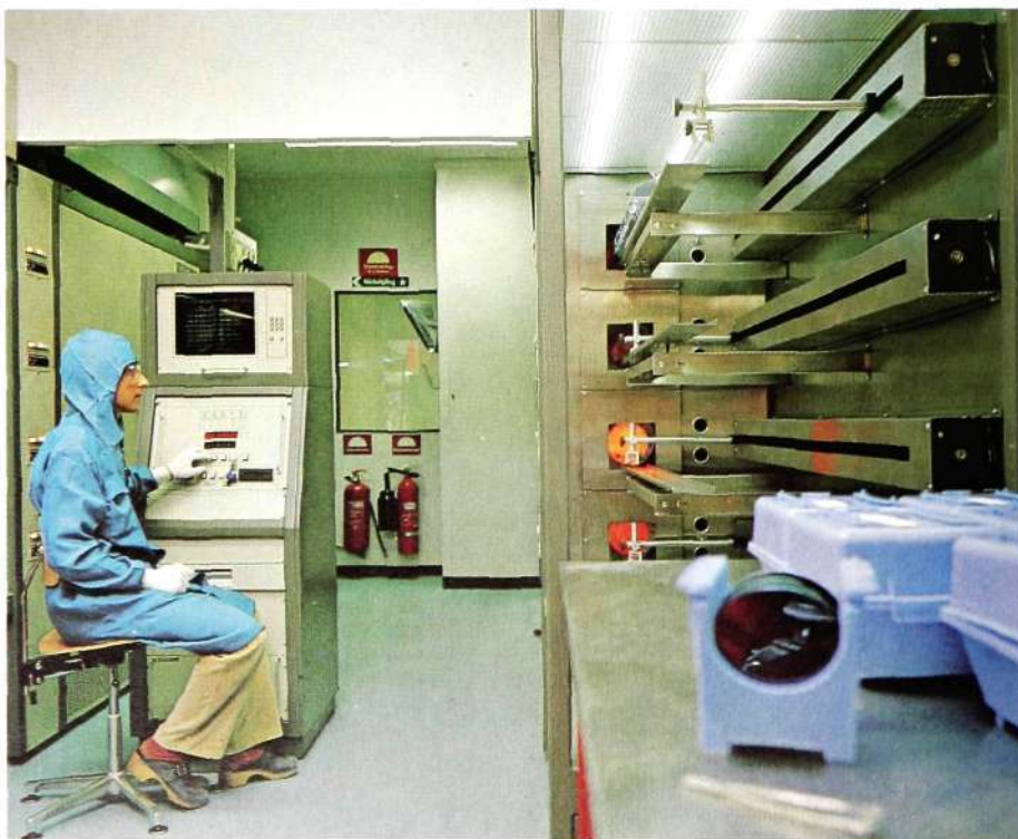
Fig. 3 Diffusion line. The wafers are fed into the oven automatically. The process is controlled by a microprocessor, to the left in the figure, which also regulates the temperature and gas flow in the oven to give a reproducible growth of oxide
