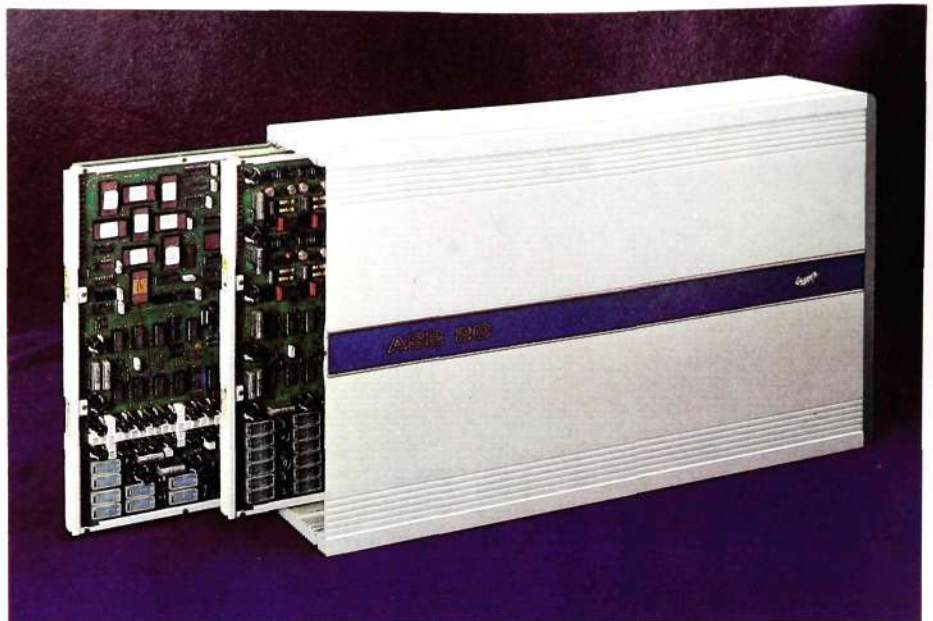
Fig. 6 The cabinet for PABX ASB 20 with two of the four printed board assemblies pulled out
