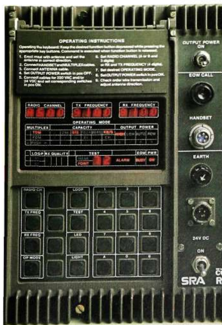
Fig. 2 The keyboard and display panel on the front of radio relay equipment CONTACT RL400
