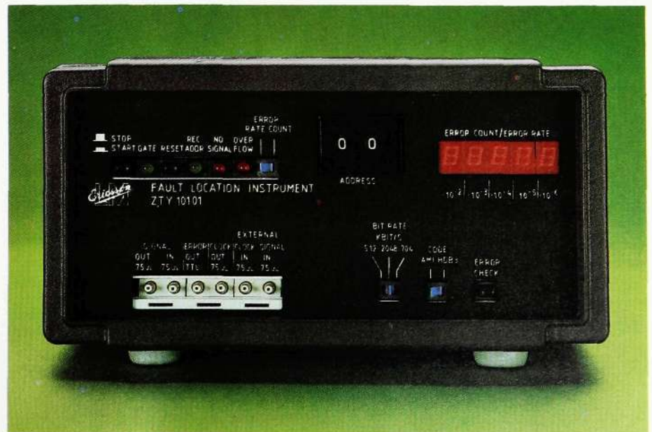
Fig. 12 Fault location instrument The front is equipped with - thumbwheel switches for addresses - error rate indicator, the rate being given by one digit - switches for selecting the bit rate, 704 or 2048 kbit/s - switches for selecting the line code, HDB3 or AMI - connectors for outgoing and incoming signals and for external instruments
