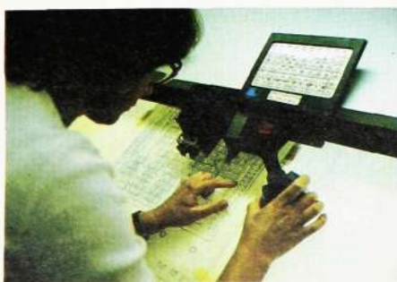
Fig. 10 Computer-aided designing of printed board assemblies at ELLEMTEL
