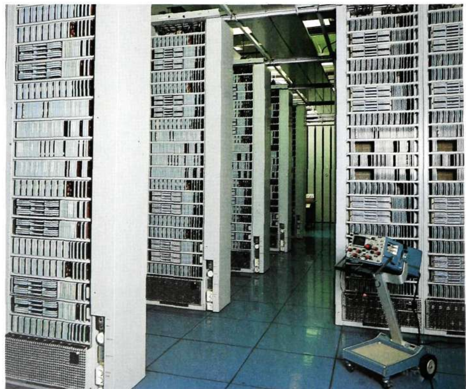
Fig. 8 Processors of type APZ 130 and APZ 150 in the MIPSC unit dealing with the AKE system
