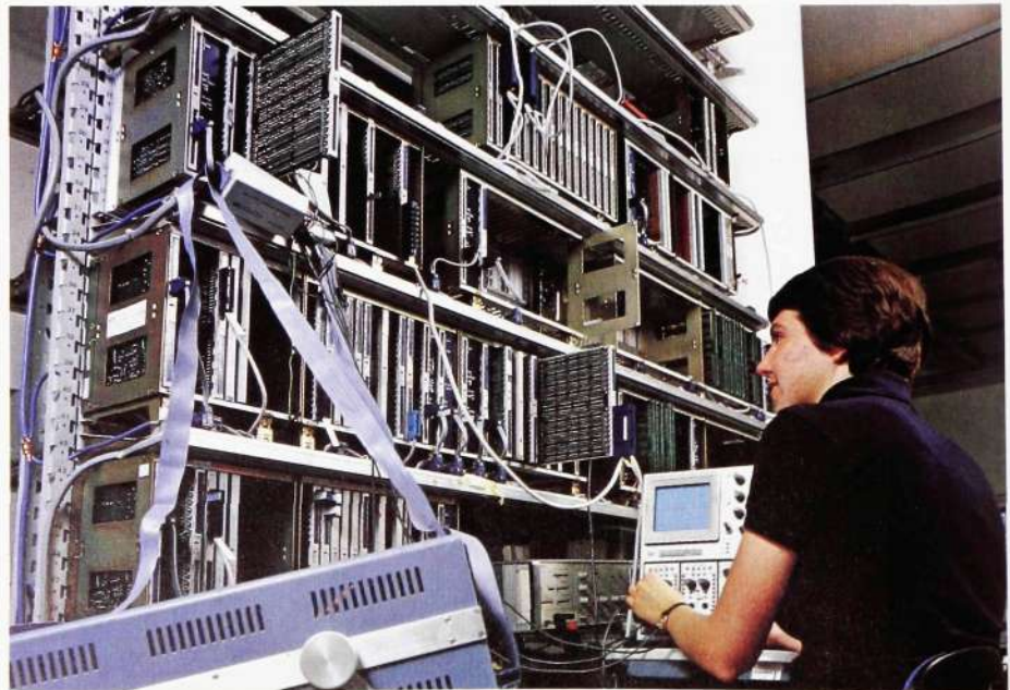
Fig. 11 Laboratory testing of the digital subscriber stage
