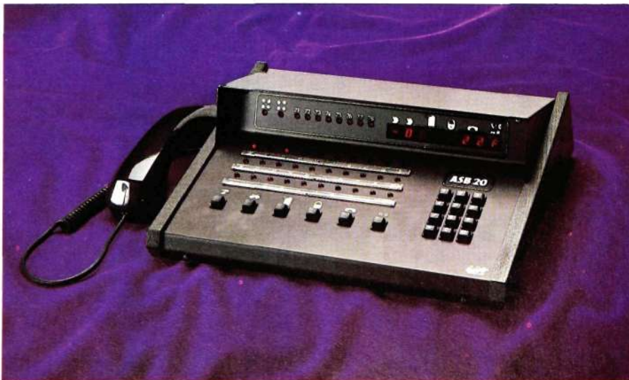
Fig. 5 The operator console in ASB 20. The upper panel contains alarm lamps, busy lamps for the trunk circuits and display with symbols for information on call progress. The lower panel contains busy lamps for the extensions, function buttons and a pushbutton unit
