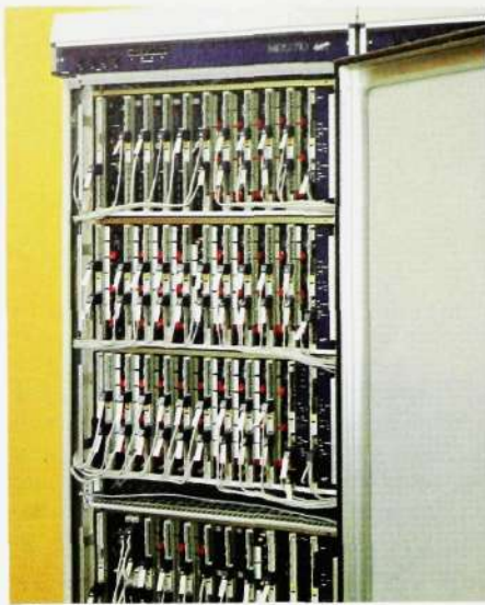
Fig. 8 MD 110, a new stored program controlled PABX for voice and data. The system has a modular structure and can be extended to 10 000 extensions
