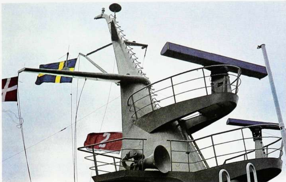
Fig. 8 A passenger ferry with radar antennas for the X and S bands. The S-band antenna is at the top
