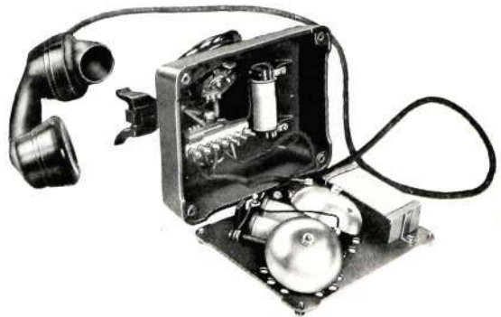
Fig. 2—View of the Interior
