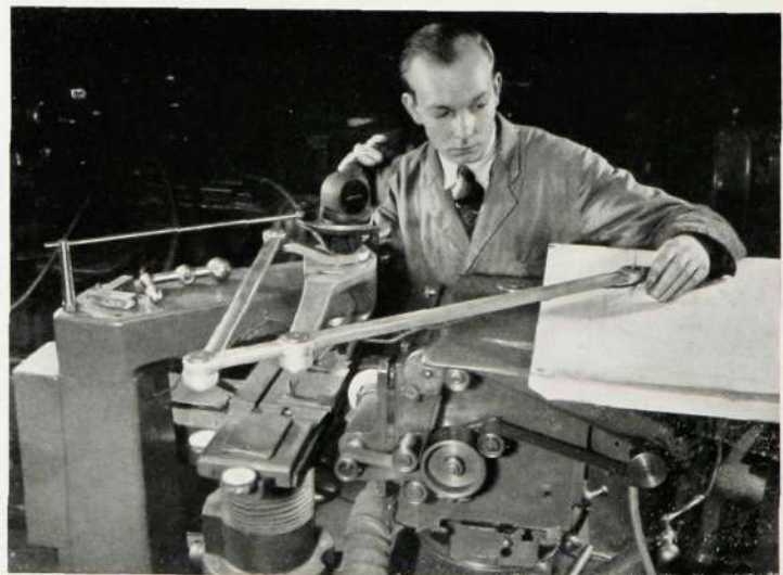
Fig. 3—Optical Profile Grinding Machine with Pantograph
