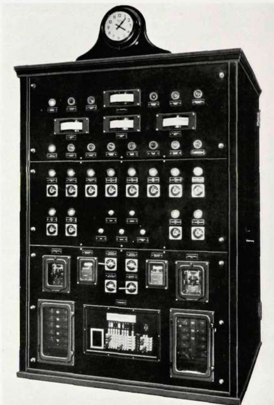
Fig. 2—Control Cabinet of the "Actadis" Transmitter
