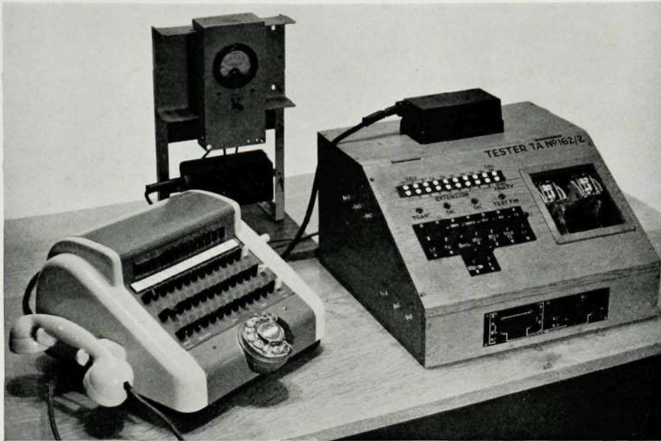
Fig. 13—Switchboard Connected for Functional Testing
