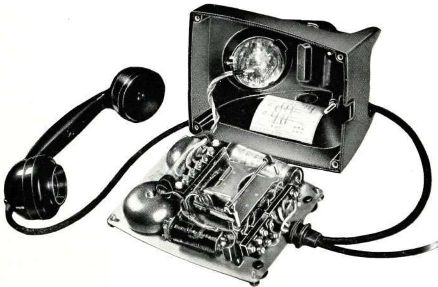
Fig. 2—Interior View of Table Telephone (Type N1025A)
