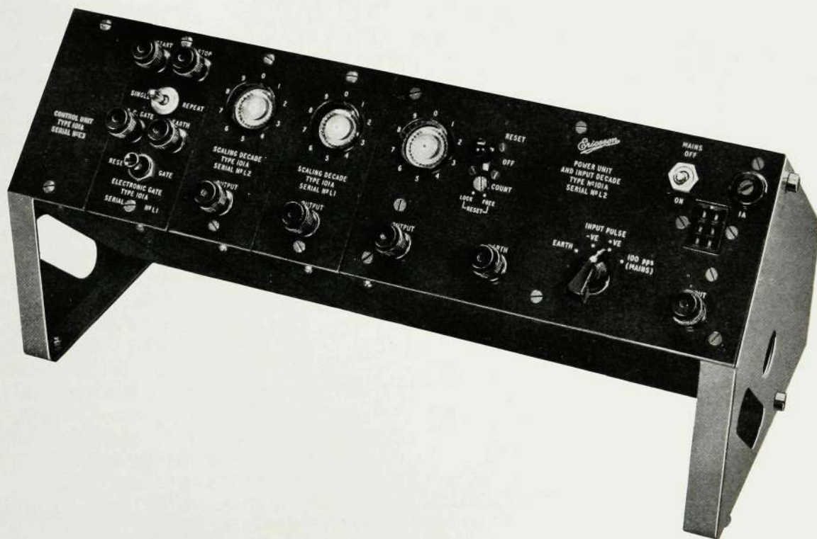
Fig. 1—Typical Assembly of Units on End Stands. The Power Unit and Input Decade is on the right
