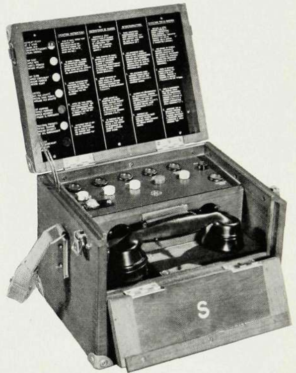
Fig. 4—Signalling Unit used on board ship when refuelling
