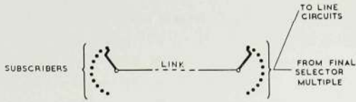
Fig. 4A—A simple Line Connector using one line circuit in the Exchange per Subscriber
