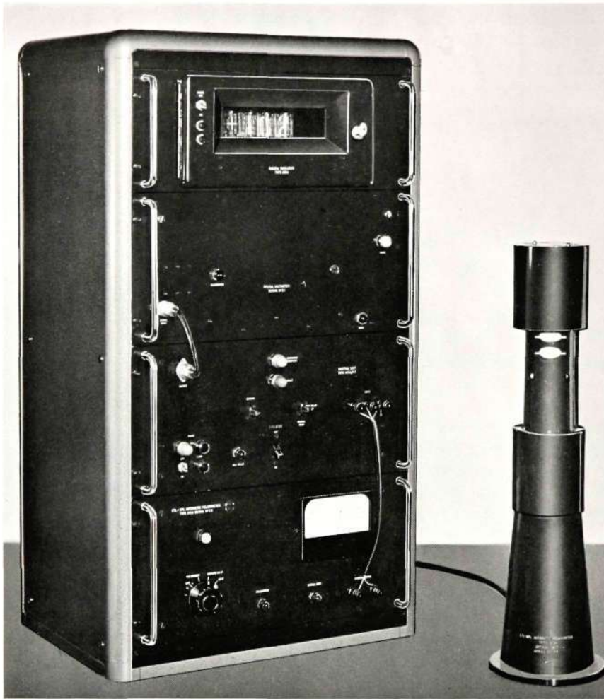
Fig 6—Automatic Polarimeter installation for British Sugar Corporation factory, Wisington
