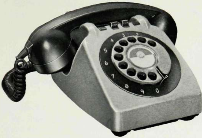
Figure 2—Non-multiple station telephone
