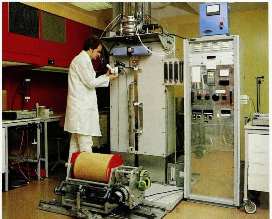
Fig. 2 Manufacture of optical fibres on a small scale in LM Ericsson's Materials Laboratory
