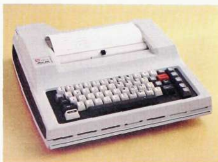
The maintenance man can, via an I/O terminal, request a printout giving the alarm class, alarm code and name and number of the faulty device
