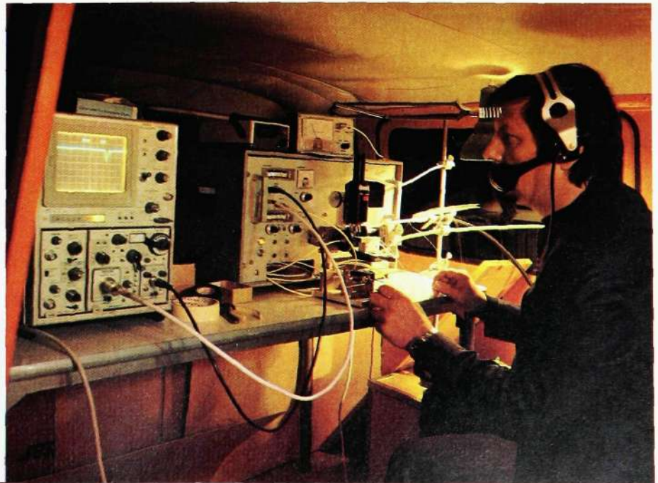
Fig. 10 Transmitter position when measuring in a cable tube
