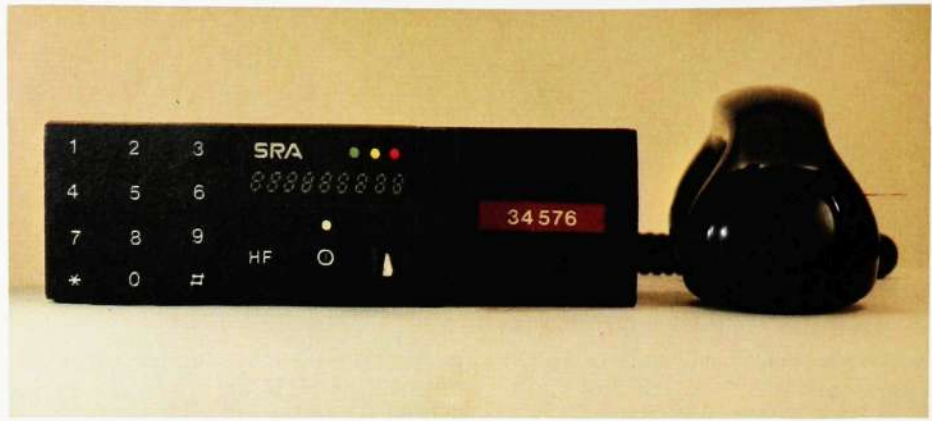
Fig. 11 A mobile telephone with a push-button set for dialling, number panel that shows the dialled number, special key HF for changeover to the loudspeaker, on-off switch and volume control. The subscriber number is shown to the right
