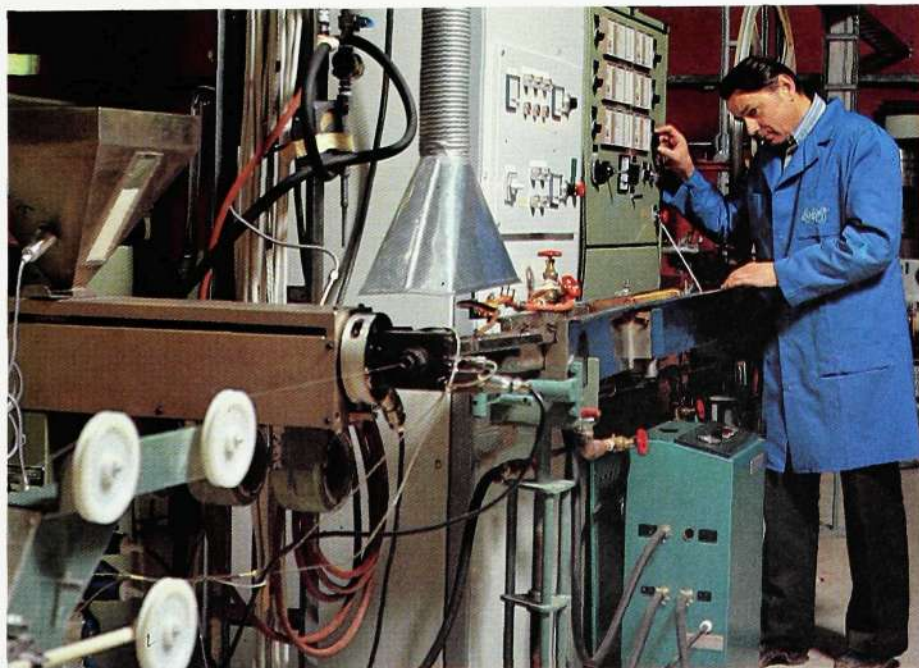
Fig. 3 Line for applying the secondary coating, with extruder and control unit
