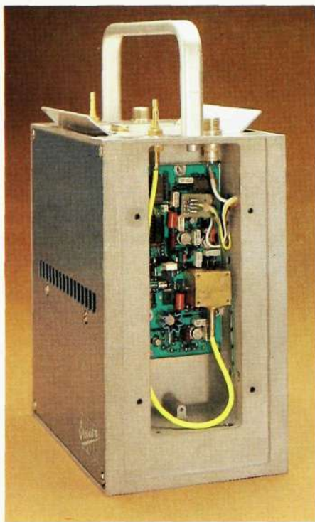
Fig. 1 Line terminal equipment ZAM 34-1 with the cover plate removed from the laser transmitter
