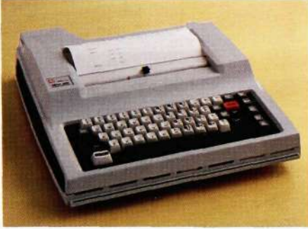
Fig. 5 I/O terminals are used in the ASB systems, for example for programming the exchange data. The terminal in the picture is portable and weighs only 5 kg
