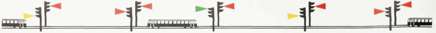
Fig. 7 Automatic block signals, controlled by track circuits, are used between stations to inform the train driver of the position of the train in front of him
