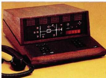
If the system detects a fault, an alarm lamp is lit in the operator's set. The operator can then order the system to indicate the alarm class and alarm code. The alarm code gives the type of device and type of fault
