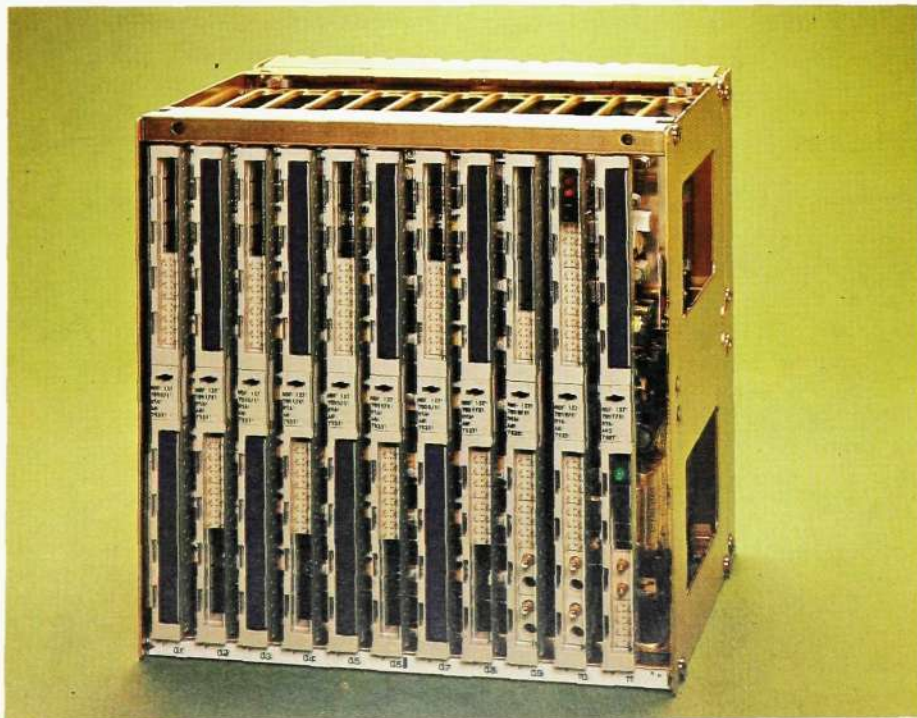
Fig. 8 ZAK 1/30-4, the PCM multiplexor equipped for 30 speech channels
