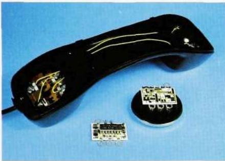
Fig. 7 Speech circuit for the DIAVOX
