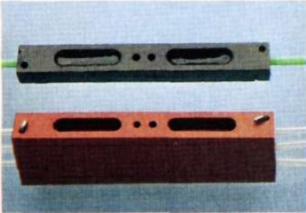
Fig. 16 Glued fibre joints. The joining pieces can be stacked on top of each other
