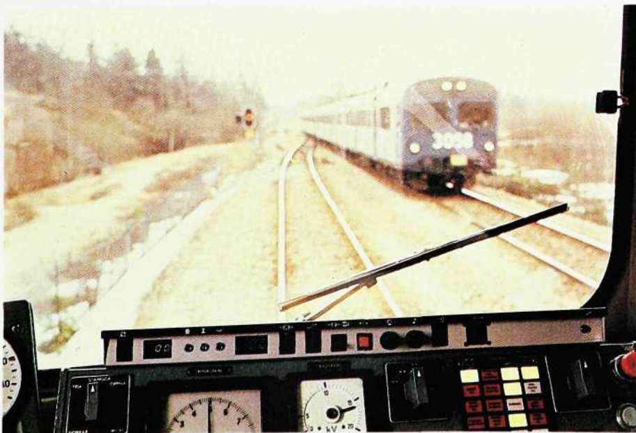
Fig. 13 The ATC system supervises that the train does not exceed the speed limits, which are depending on the train itself, the condition of the track and the traffic situation
