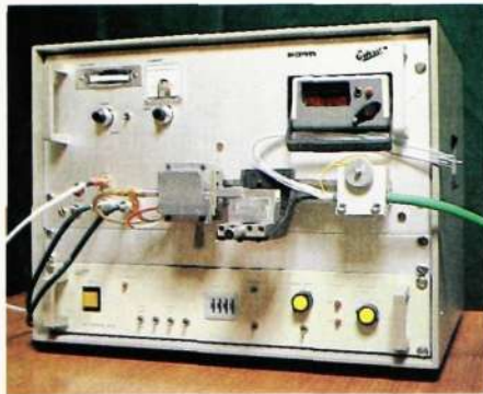
Fig. 8 Equipment for measuring attenuation and dispersion Top: Transmitter Bottom: Receiver
