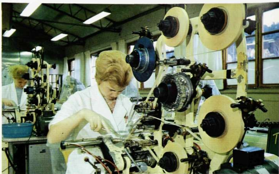
Fig. 10 Winding of capacitors. The machines were designed and manufactured by RIFA
