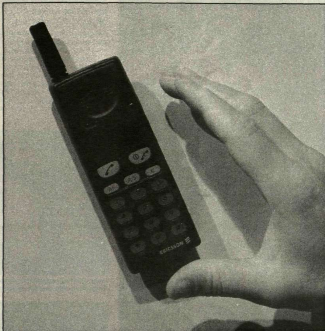
With a weight of only 200 grams the EH 237 is the market's smallest pocket phone. The length is 130 millimeters.
