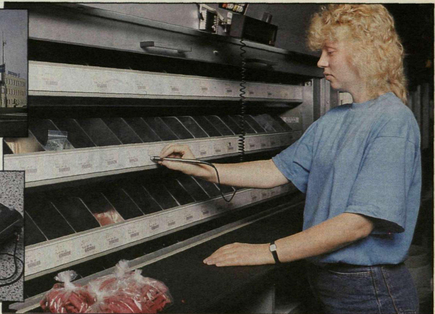
All goods handling is done automatically. To gather up material for an order bar code handling is used, which registers and later follows the entire process through to manufacturing. Above, Trea Kuipers-Hoving gathers up material for an order.
