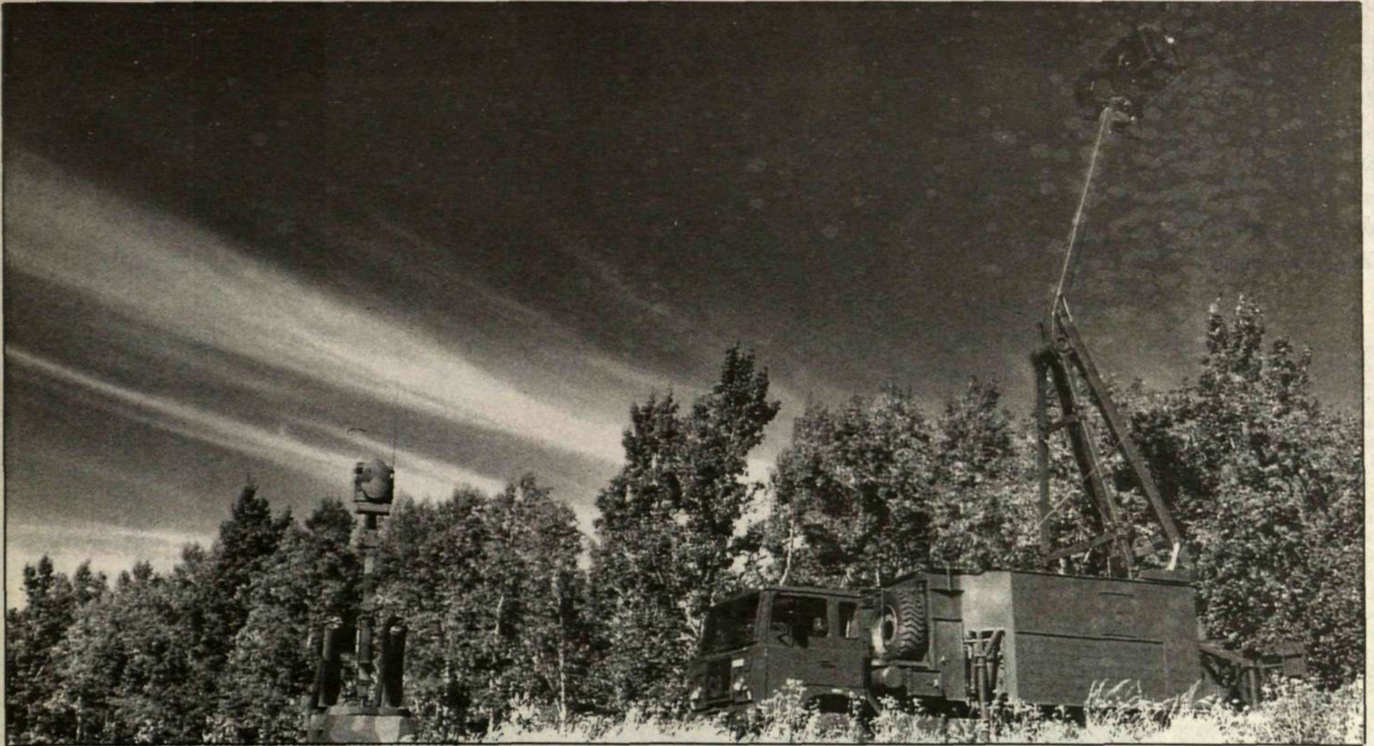
BAMSE consists of an intelligence unit with surveillance radar (ERE's GIRADDE 3D, right in the picture) and a firing unit, which ERE equips with a companion radar as well as parts of missile-guiding electronics.
