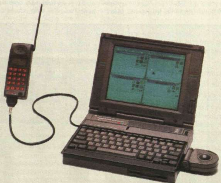
Texas TravelMate notebook computer with Ericsson modem connected to an Ericsson handheld mobile phone NH 97.
