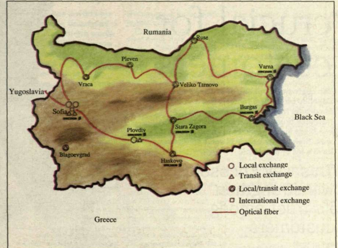
BULGARIA'S DIGITAL TELE NETWORK. The new digital tele network in Bulgaria lies around two nationwide fiberoptic rings. Ericsson works with transit and local exchanges in the southern part of the country. Illustration: Gunnar Englund
