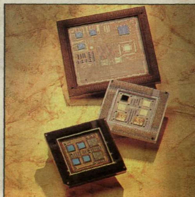
Multi-chip modules (MCMs) provide high packaging densities for advanced microelectronic products.
