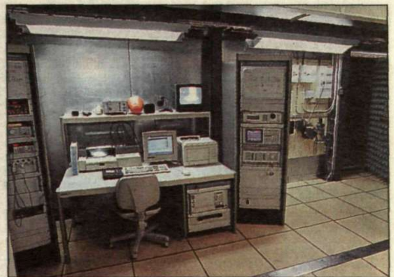
Testing is directed from the control room. Using a computer, it is possible to create various types of energy fields around the object being tested and observe how it reacts in a given situation.
